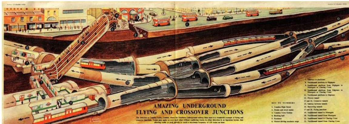
Figure 17: Multilevel tunnelling description [23]
