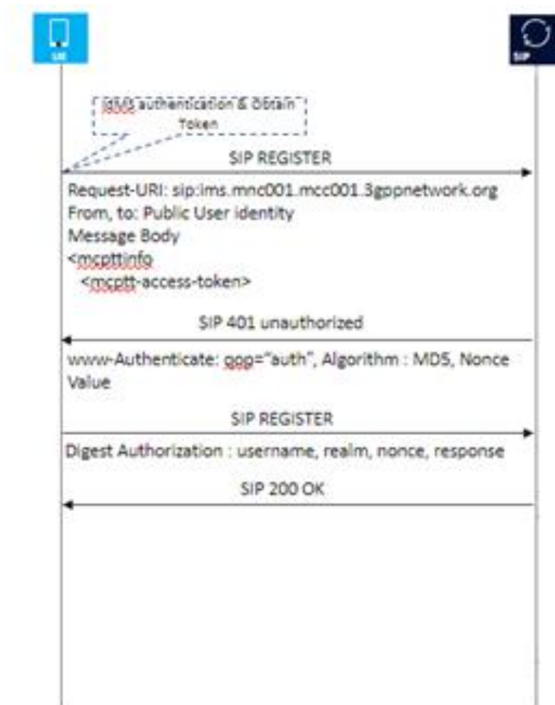
Figure 7: SIP Registration call flow (Ref. D3.3v2)
