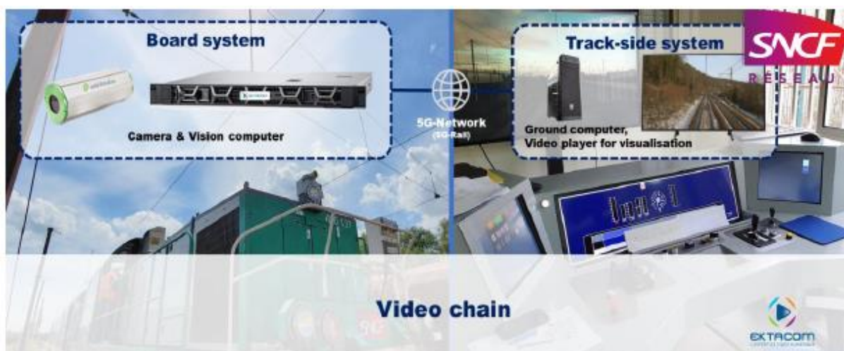
Figure 34: Presentation of remote vision Video chain (Ref. D5.1)
