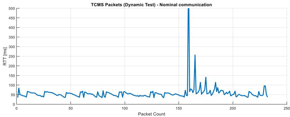
Figure 89: RTT for TCMS Dynamic Test 1/2, Test Case No. TCMS\_TC\_001 (TC\_001b) (Testbed Germany)
