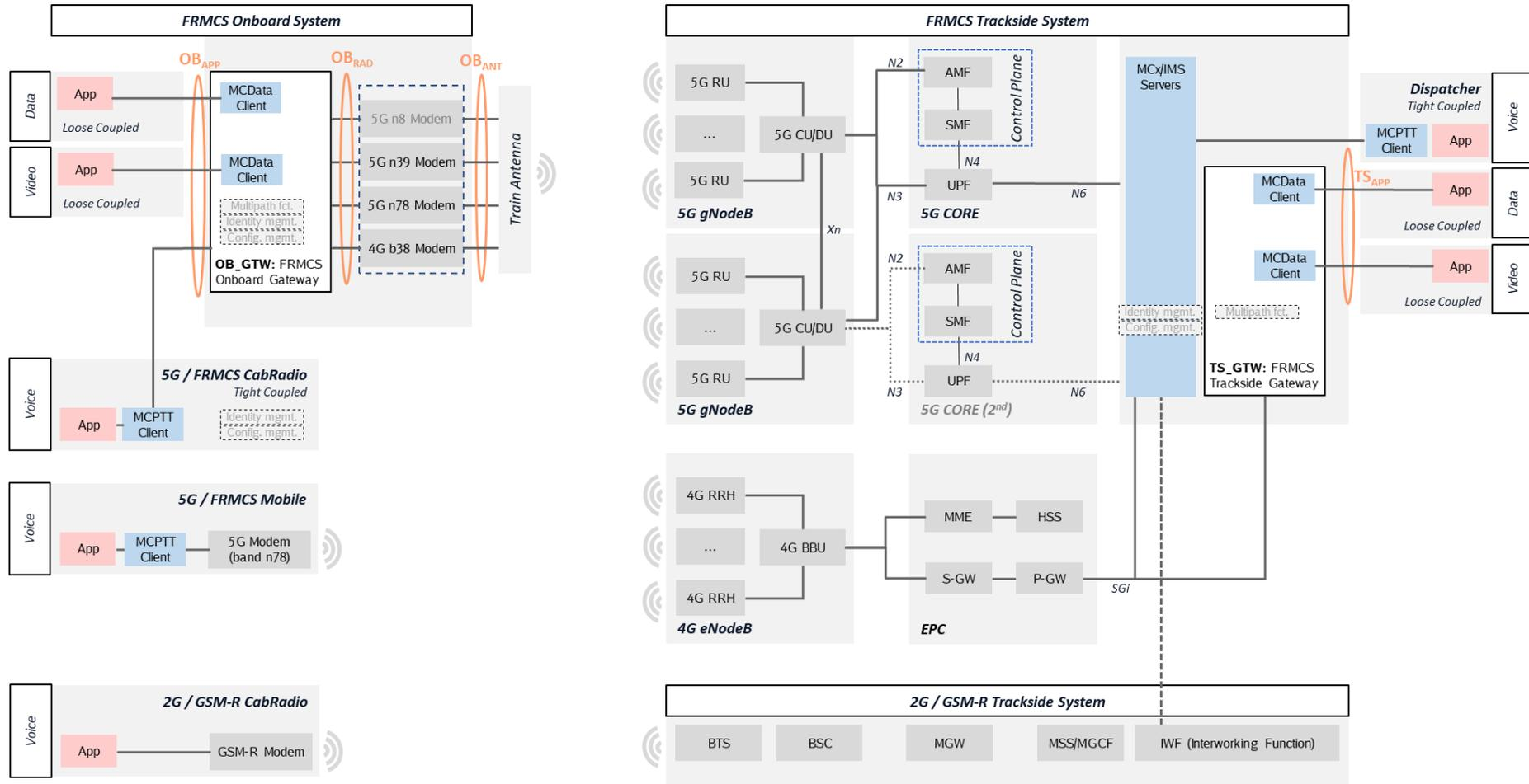
Figure 38: Common end-to-end test architecture of WP5 to perform the functional and performance tests of the FRMCS system.
