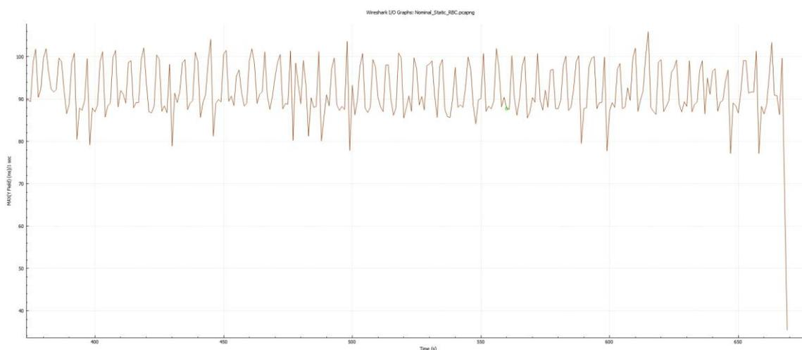
Figure 62: RTT for ETCS Static Tests, captured in trackside traces (RBC), Test Case No. ETCS\_WP3-WP5\_TC\_001 (Testbed Germany)
