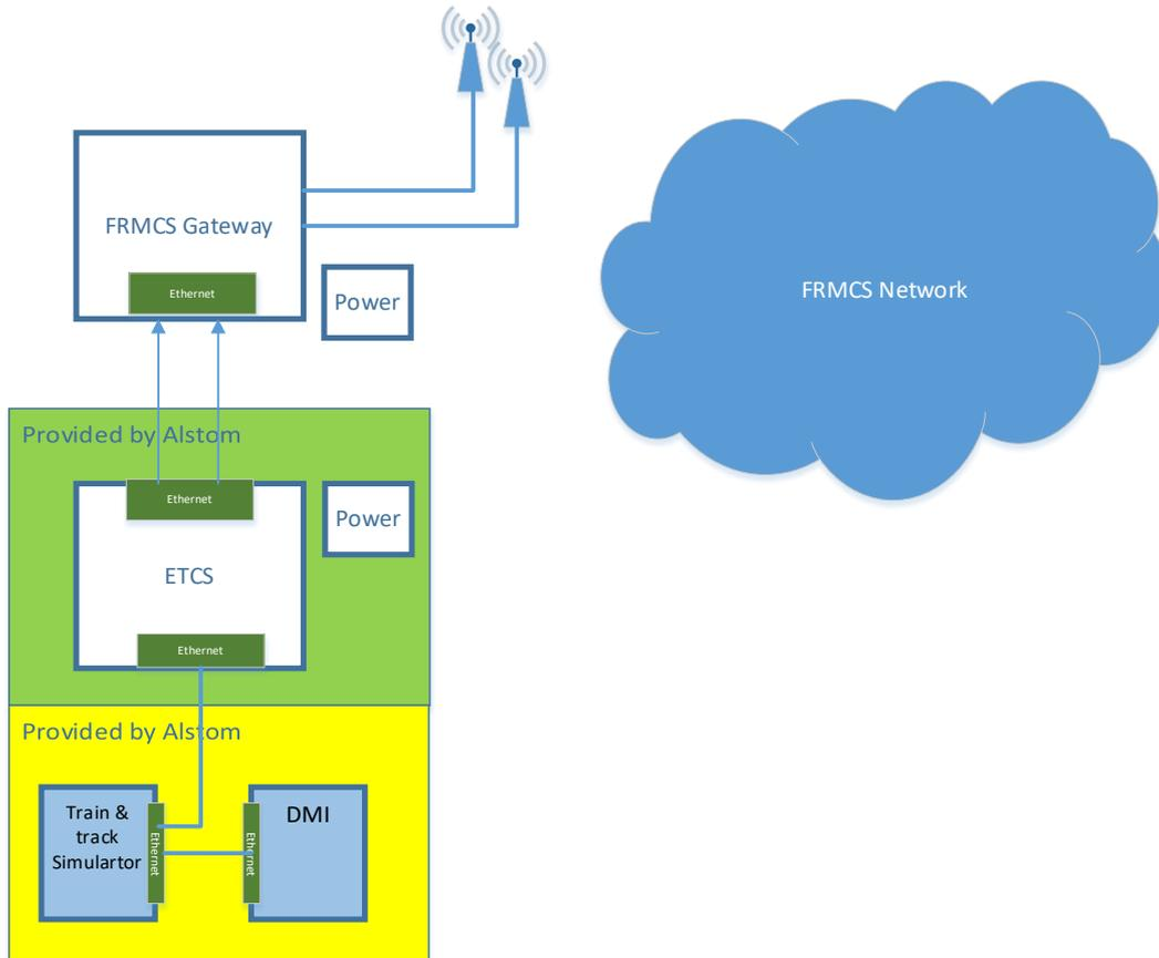
Figure 35: On-board design for ETCS/ATP over FRMCS tests (Testbed France)
