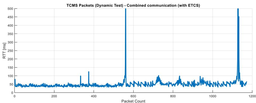
Figure 90: RTT for TCMS Dynamic Test 2/2, Test Case No. TCMS\_TC\_001 (TC\_001b) (Testbed Germany)
