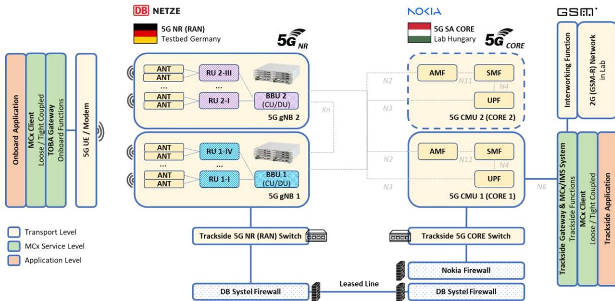
Figure 5: End-to-end network realization in the Testbed Germany
