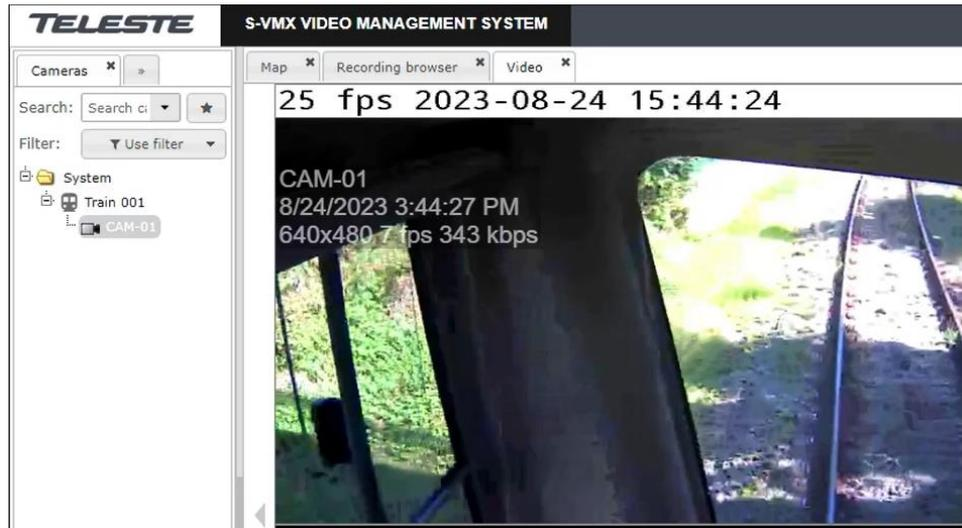
Figure 106: VGA Video Streaming Drive Test (Testbed Germany), showing short quality degradation during an inter-gNB handover situation
