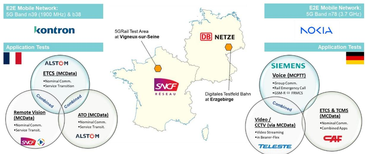
Figure 1: Location and scope of 5GRAIL Testbed in France and Germany
