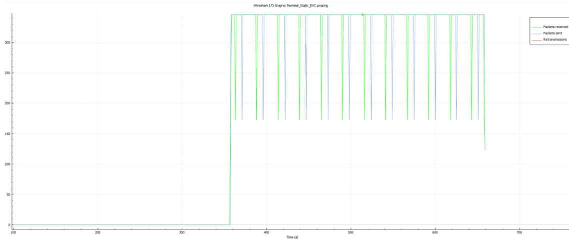
Figure 61: Packet Information (Sent/Received/Retransmissions) for ETCS Static Tests, captured in onboard traces (EVC), Test Case No. ETCS\_WP3-WP5\_TC\_001 (Testbed Germany)
