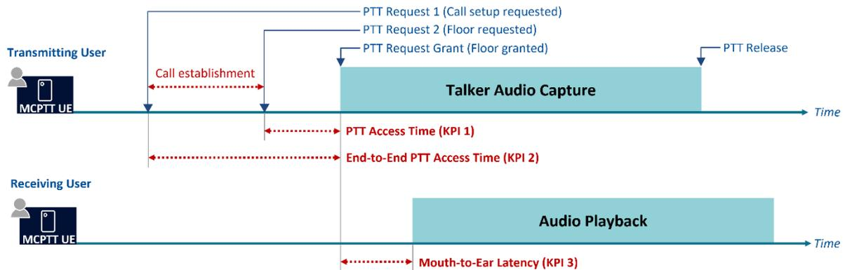
Figure 41: KPIs for MCPTT measurements in voice applications acc. to 3GPP TS 22.179
