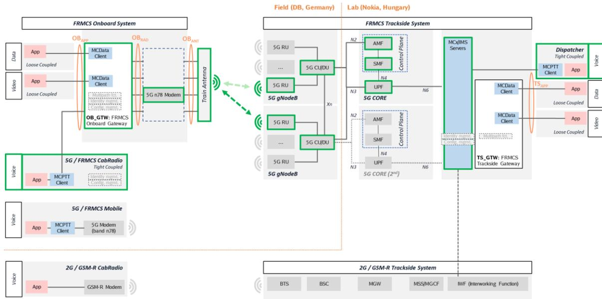
Figure 43: Architecture for test case Voice\_019, with intra- and inter-gNodeB handover (Testbed Germany)
