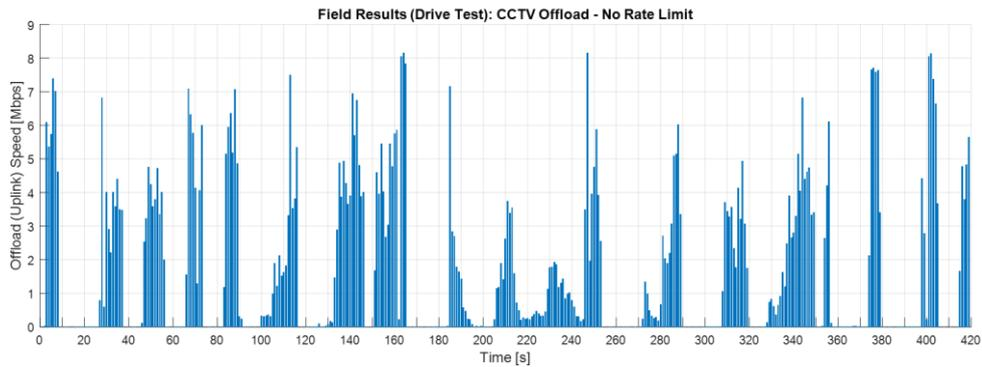
Figure 111: CCTV Offload performance in a dynamic setup (7 min drive test) without offload speed limitation, Test Case No. CCTV\_TC\_001
