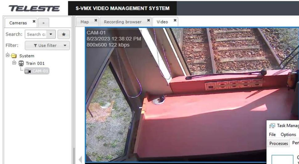
Figure 98: SVGA Video Streaming Stationary Test (Testbed Germany), snapshot with unexpected quality degradation (122 kbps)
