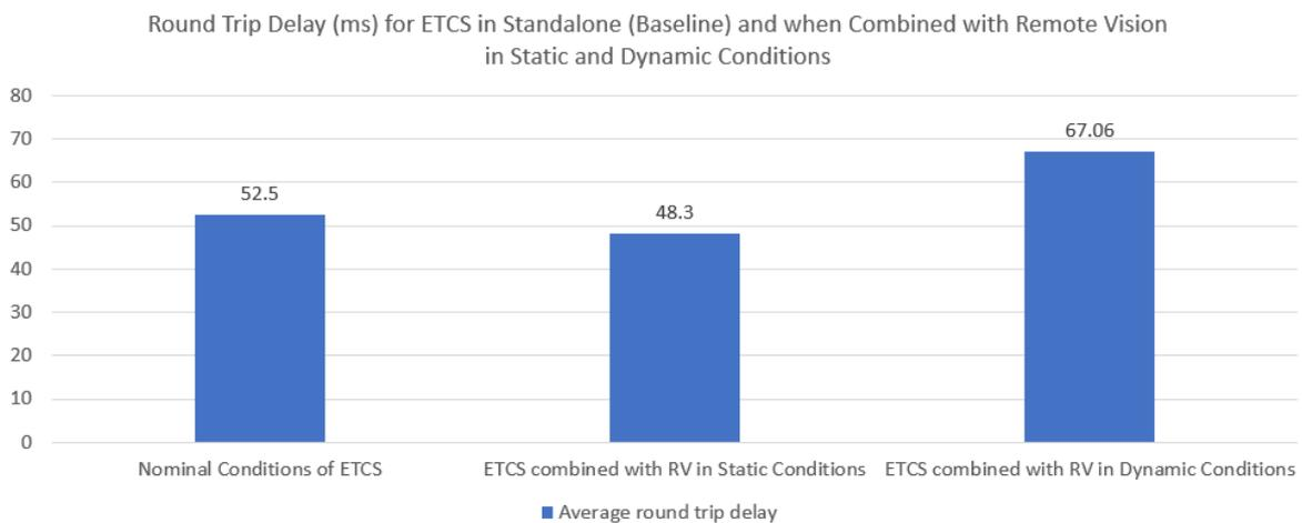
Figure 141: Average Round Trip Delay [ms] benchmarking for ETCS and Remote Vision (Testbed France)
