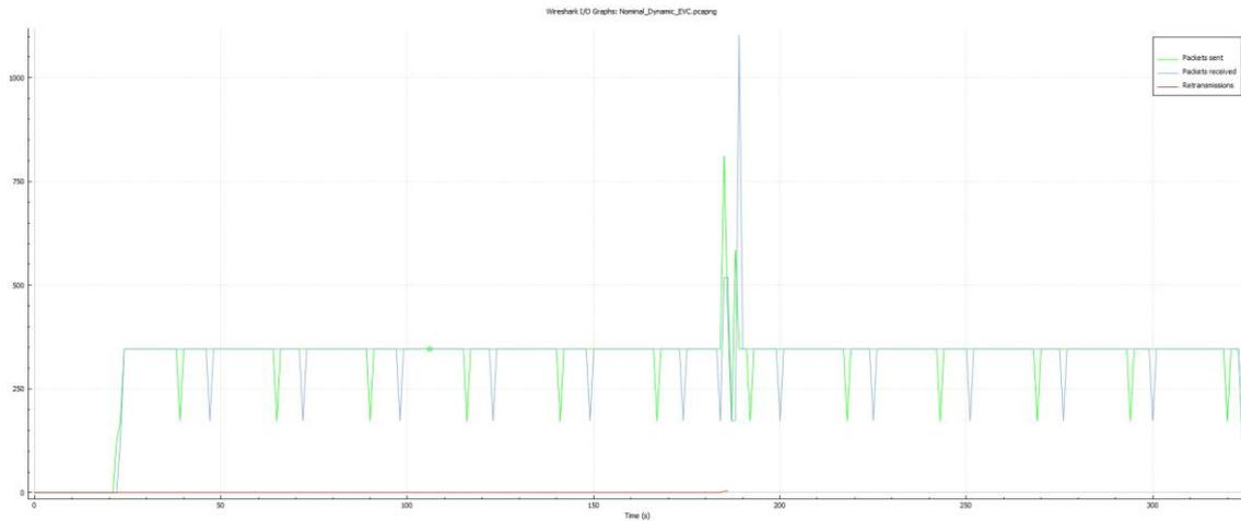
Figure 65: Packet Information (Sent/Received/Retransmissions) for ETCS Dynamic Tests, captured in onboard traces (EVC), Test Case No. ETCS\_WP3-WP5\_TC\_005 (Testbed Germany)
