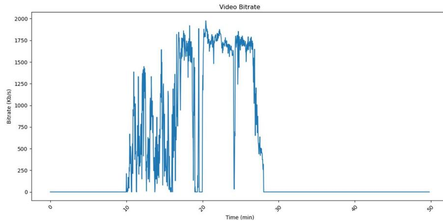
Figure 133: Fluctuating bitrate from the RV application metrics (adaptation in codecs)
