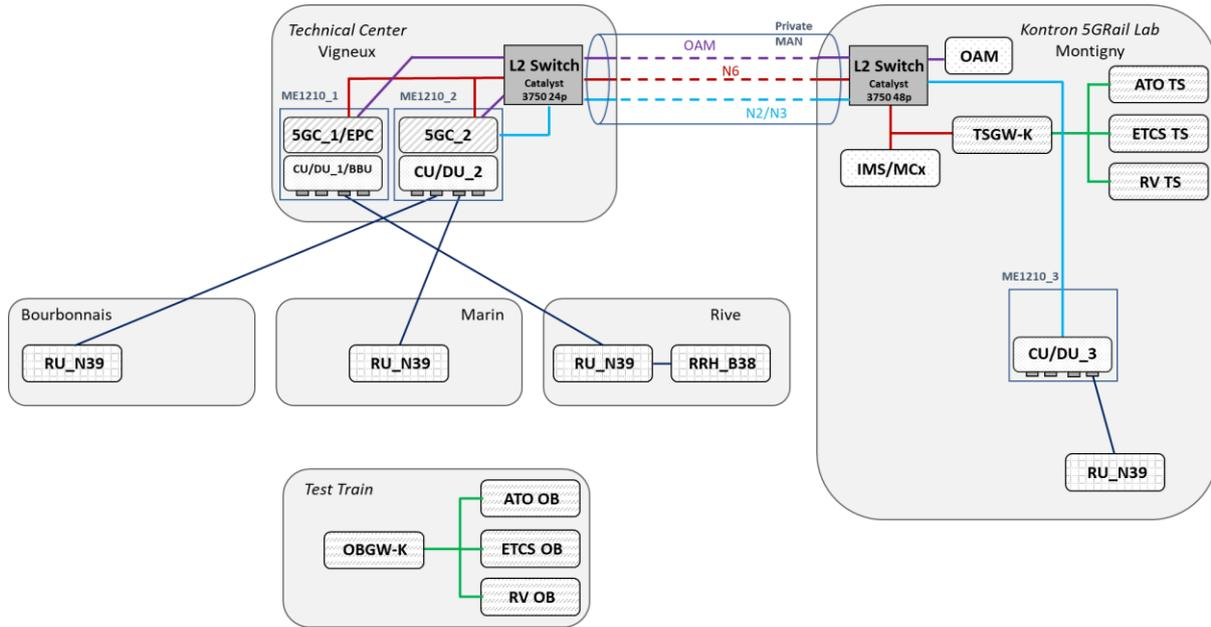
Figure 28: 5G (and 4G) network realization and interconnection of sites in the 5G RAIL Testbed France
