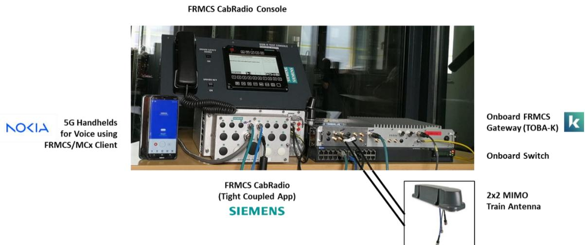
Figure 14: Example of the on-board equipment setup used for voice tests (Testbed Germany)
