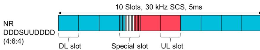
Figure 143: Example of a 5G NR TDD frame pattern with DL, UL and Special slots
