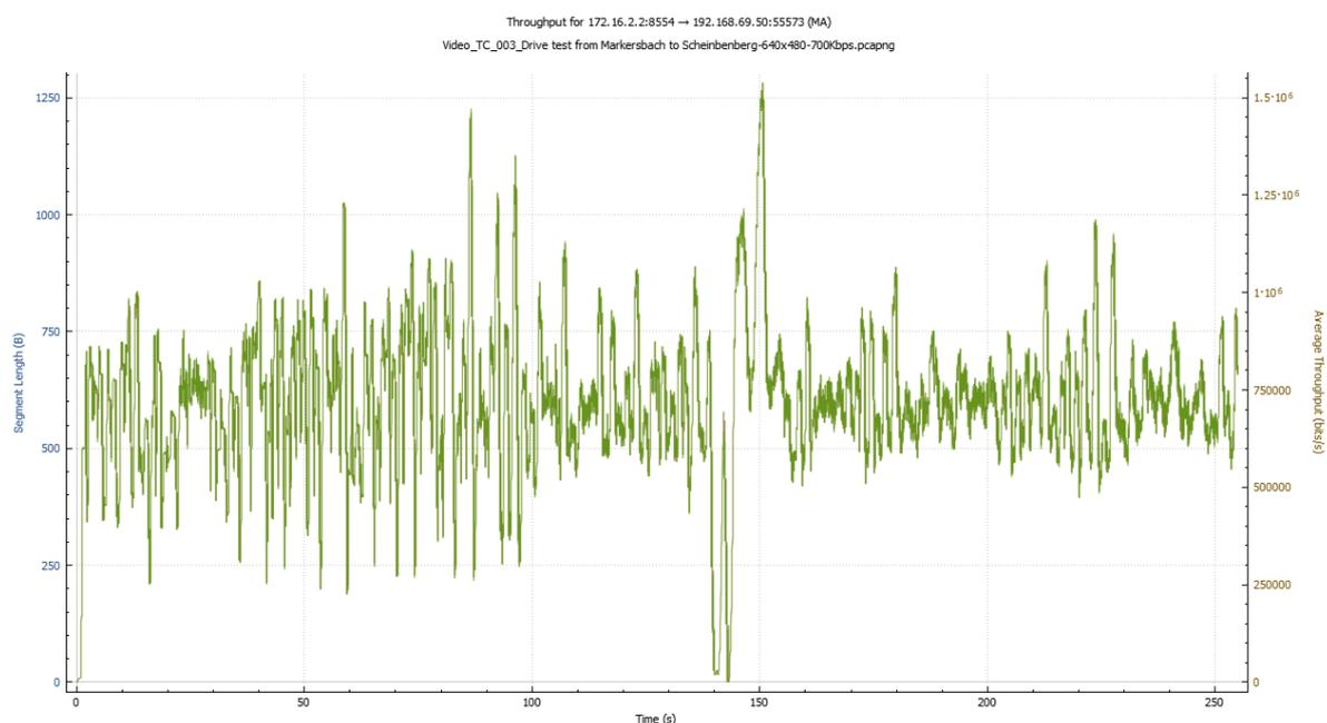
Figure 107: VGA Video Streaming Drive Test (Testbed Germany), throughput / goodput over time, Test Case No. Video\_TC\_003
