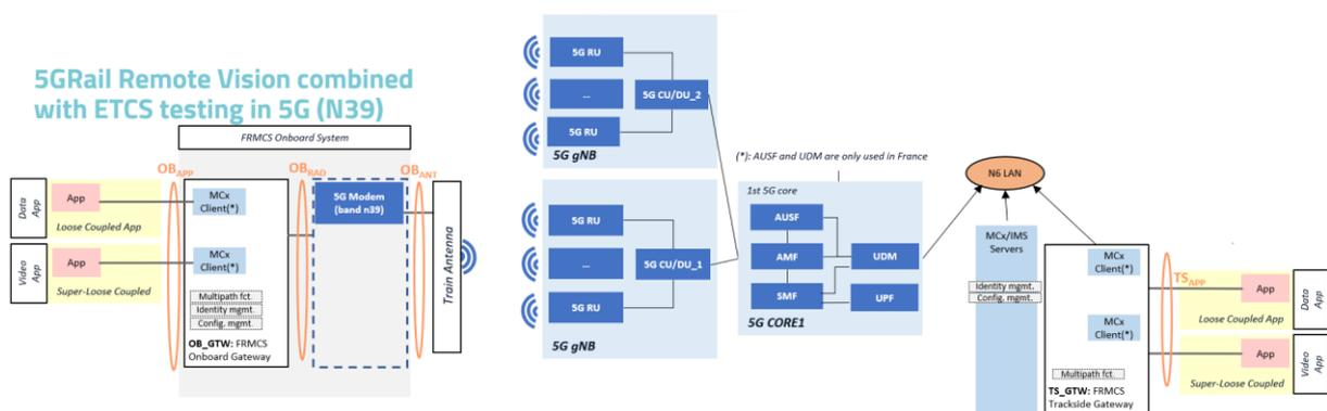
Figure 138: Involved Building blocks when testing Remote Vision combined with ETCS application (Testbed France)
