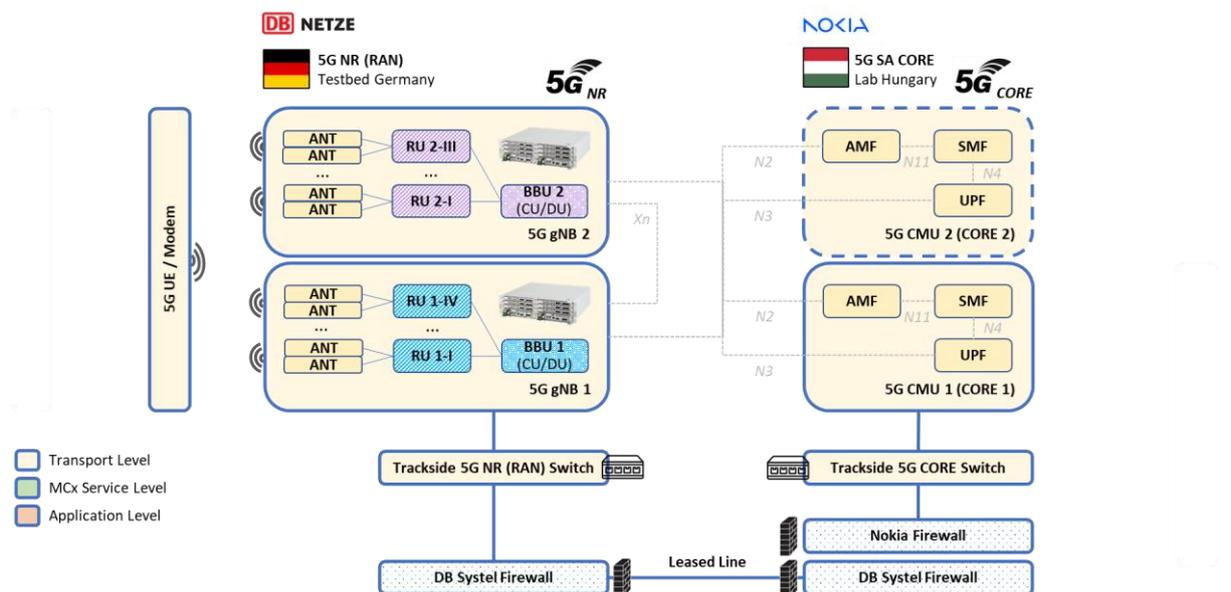
Figure 4: 5G SA network realization in the Testbed Germany with onsite 5G Radio and remote 5G Core
