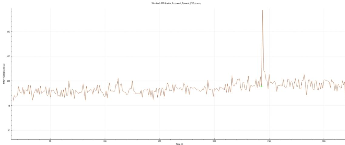
Figure 72: RTT for ETCS Dynamic Tests with increased traffic, captured in onboard traces (EVC), Test Case No. ETCS\_WP3-WP5\_TC\_003 (Testbed Germany)
