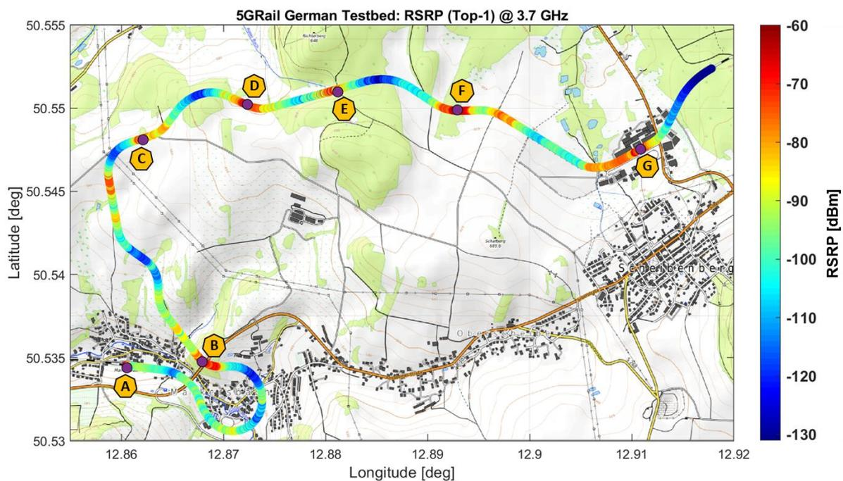
Figure 16: RSRP along the test track (Testbed Germany)
