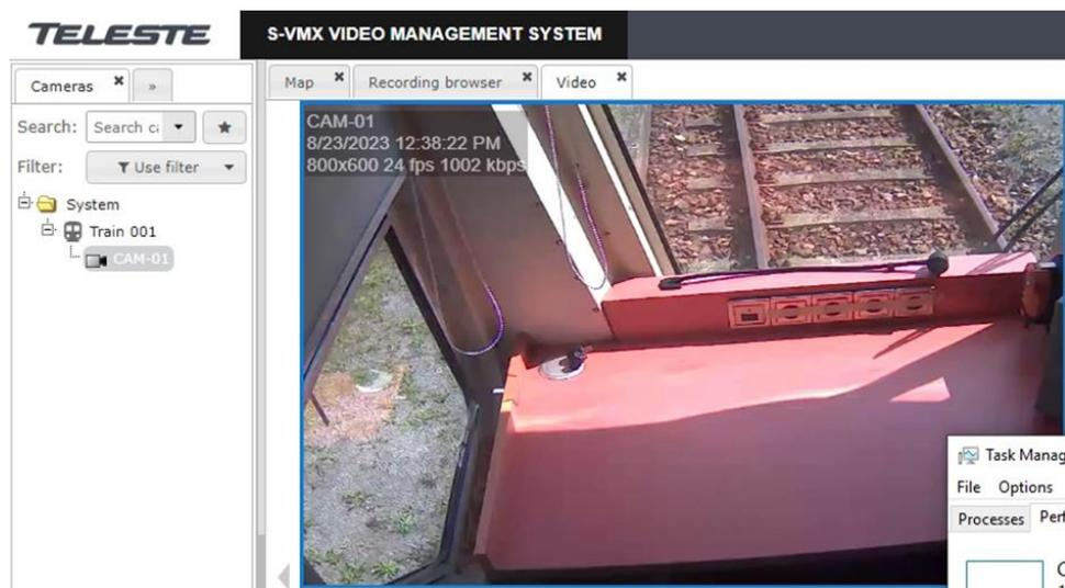
Figure 97: SVGA Video Streaming Stationary Test (Testbed Germany), snapshot with good quality (24 fps, 1002 kbps)
