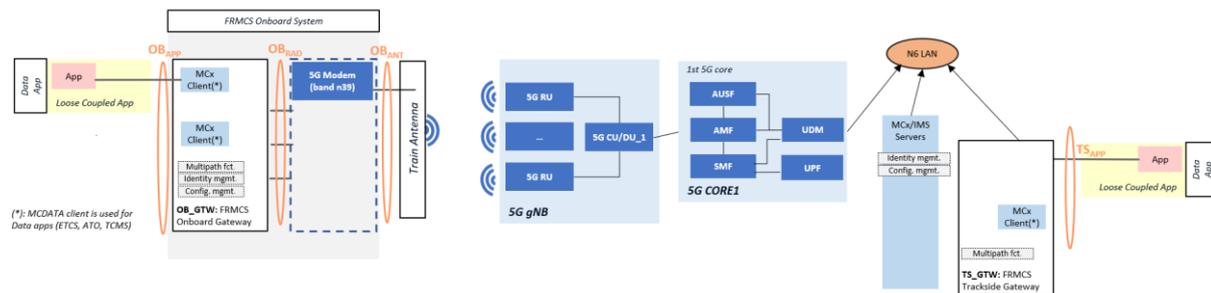
Figure 114: Involved building blocks when testing nominal communication in ETCS L2 (Testbed France)
