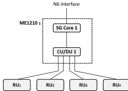
Figure 120: Configuration for intra gNodeB HO under the same 5G Core (Ref.D4.2 [10])
