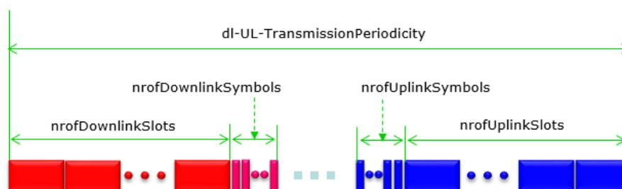
Figure 144: Definition of TDD UL-DL slot configuration by 3GPP
