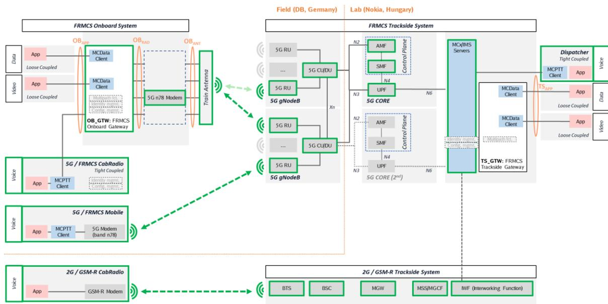
Figure 46: Architecture for test case Voice\_021 (Testbed Germany)
