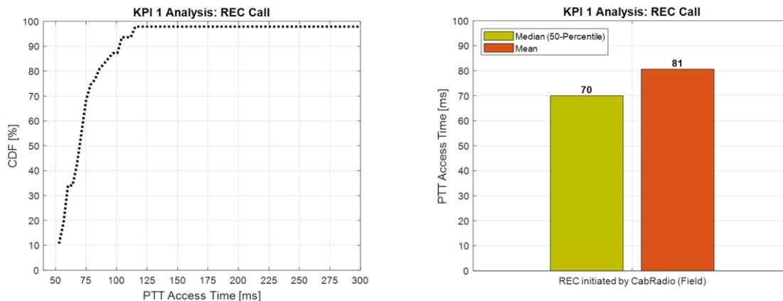
Figure 52: Statistical analysis of PTT Access Times for MCPTT railway emergency calls (Testbed Germany)
