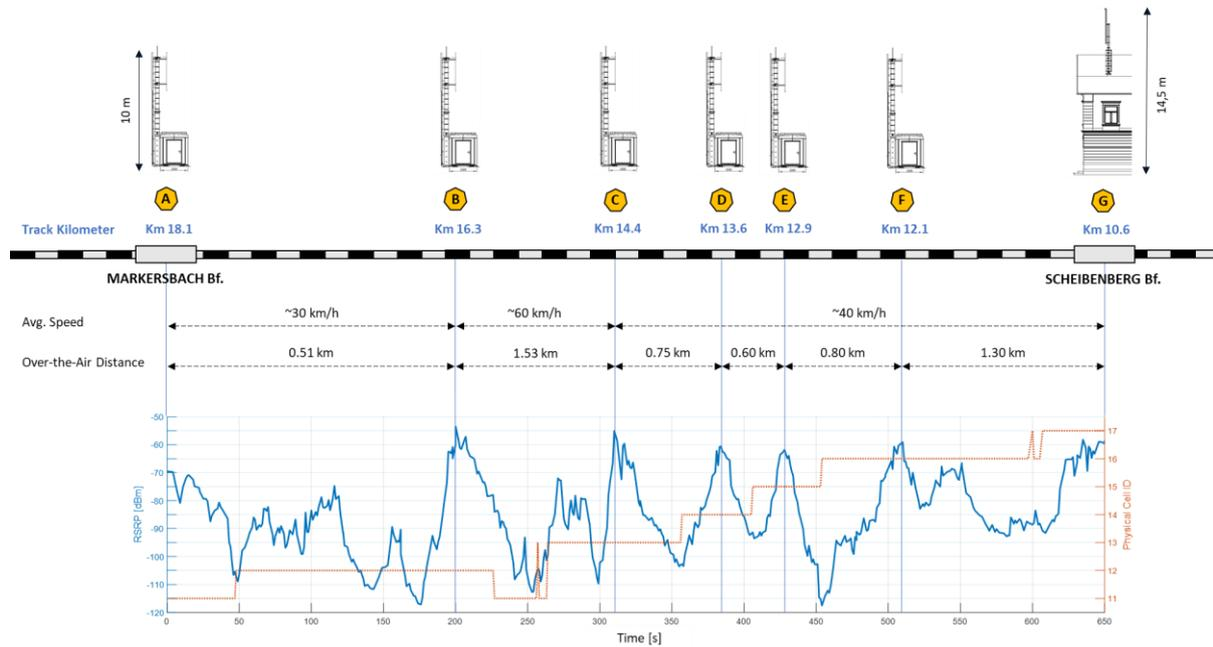
Figure 15: Observed RSRP and Cell IDs during a drive test (Testbed Germany)
