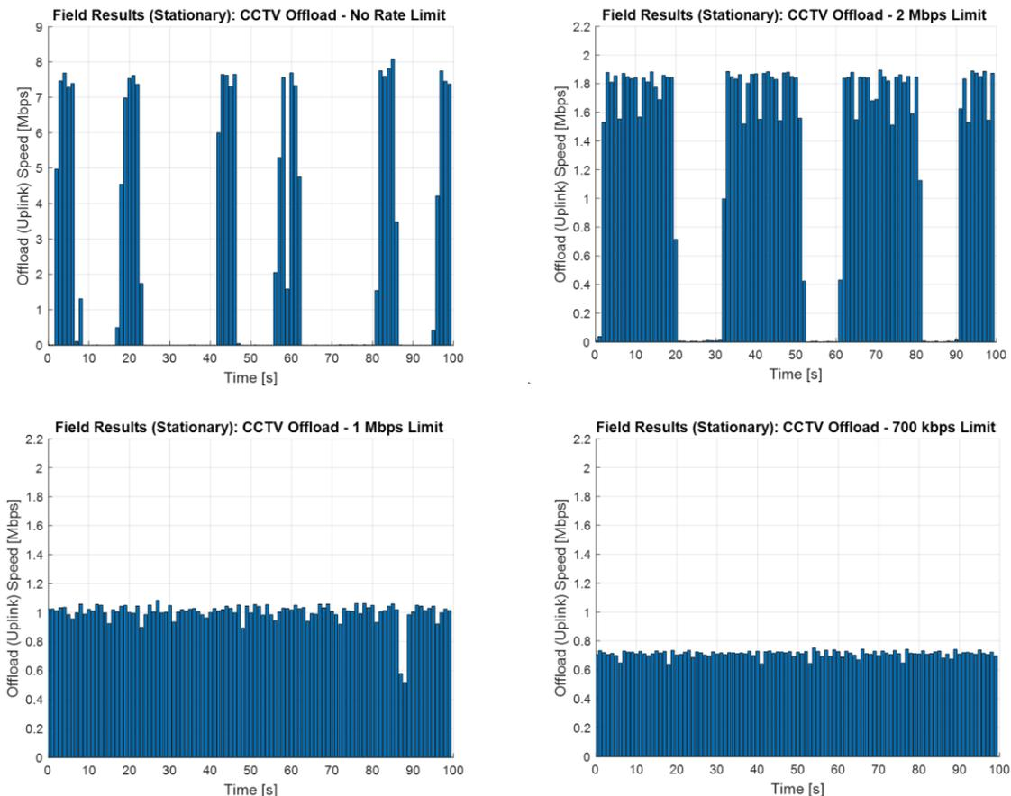
Figure 110: CCTV Offload performance in a stationary setup with different offload speed limitations, Test Case No. CCTV\_TC\_001
