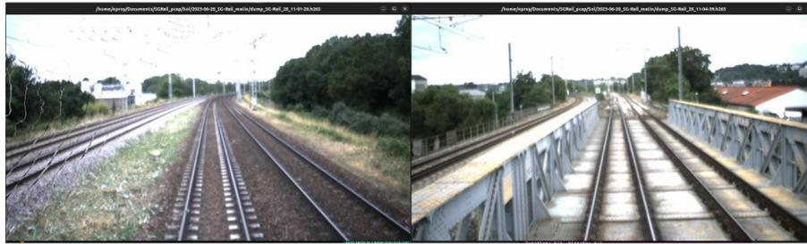
Figure 132: Impressions of remotely viewed images (Over-exposure on camera)
