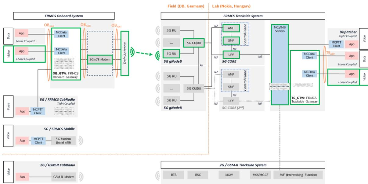
Figure 93: Architecture for test case Video\_TC\_001 (Testbed Germany)
