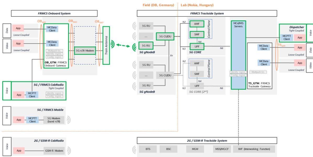
Figure 42: Architecture for test cases Voice\_008 and Voice\_009 (Testbed Germany)
