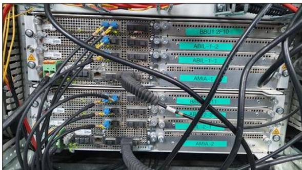
Figure 8: 2x 5G CU/DU in Testbed Germany
