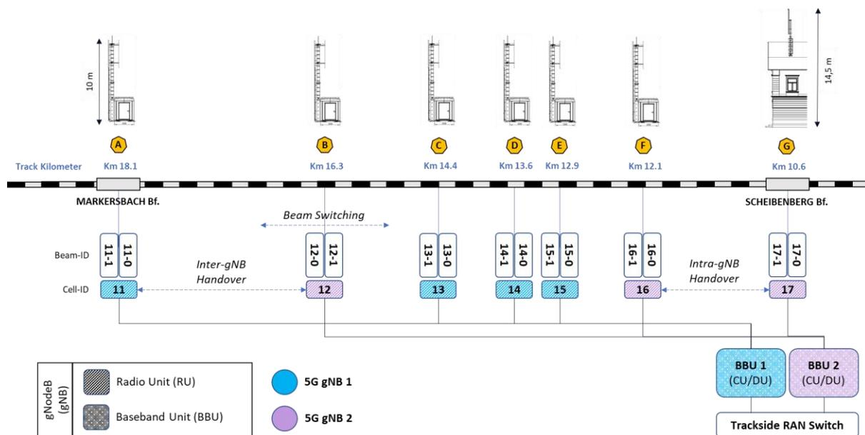
Figure 10: Handover characteristics of the 5G radio access network RAN in the Testbed Germany
