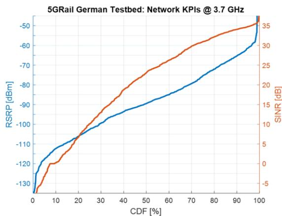
Figure 18: CDFs of RSRP and SINR (Testbed Germany)
