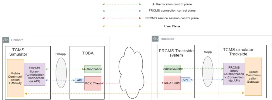
Figure 57: TCMS prototype architecture (provided by CAF)
