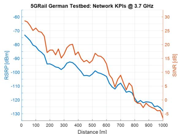
Figure 19: RSRP and SINR over Distance (Testbed Germany)
