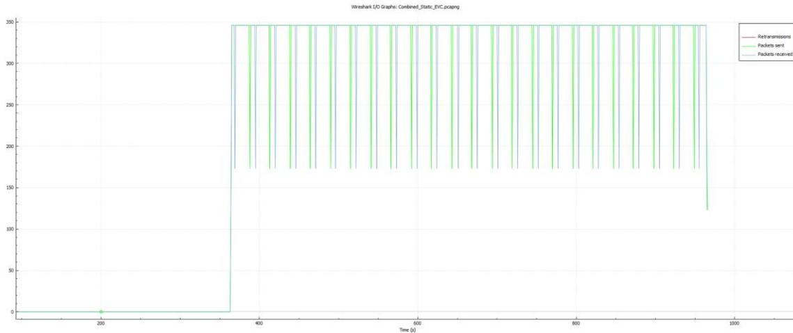
Figure 79: Packet Information (Sent/Received/Retransmissions) for ETCS in Combined Application Static Tests, captured in onboard traces (EVC), Test Case No. ETCS\_WP3-WP5\_TC\_004 (Testbed Germany)
