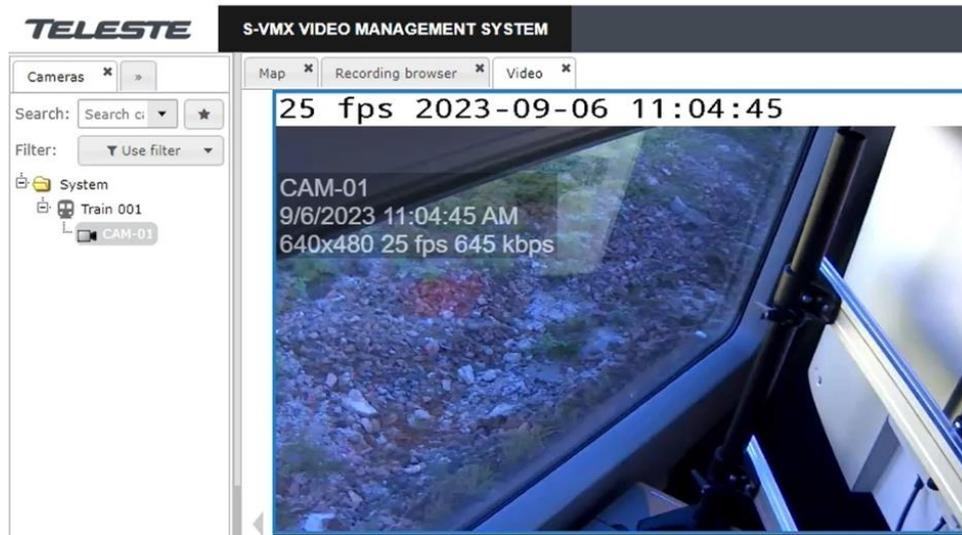
Figure 103: VGA Video Streaming Stationary Test (Testbed Germany), latency test showing same time stamps of onboard computer (transmitter side) and trackside server (receiver side), Test Case No. Video\_TC\_001
