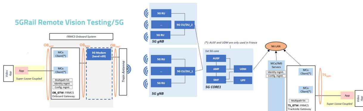
Figure 129: Involved Building blocks when testing Remote Vision as a Stand-Alone Application (Testbed France)
