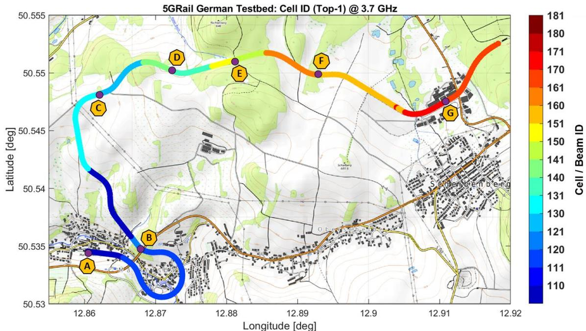
Figure 17: Cell IDs ('XX') and Beam IDs ('Y') in format 'XXY' along the test track (Testbed Germany)
