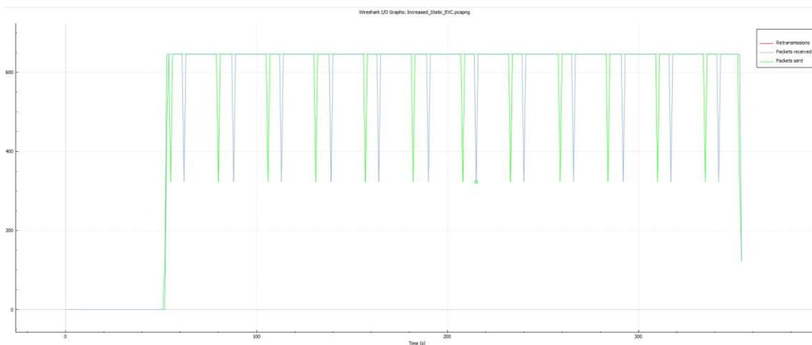
Figure 69: Packet Information (Sent/Received/Retransmissions) for ETCS Static Tests with increased traffic, captured in onboard traces (EVC), Test Case No. ETCS\_WP3-WP5\_TC\_003 (Testbed Germany)
