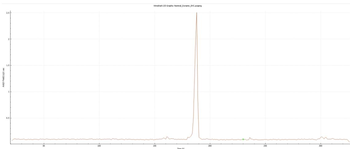
Figure 64: RTT for ETCS Dynamic Tests, captured in onboard traces (EVC), Test Case No. ETCS\_WP3-WP5\_TC\_005 (Testbed Germany)
