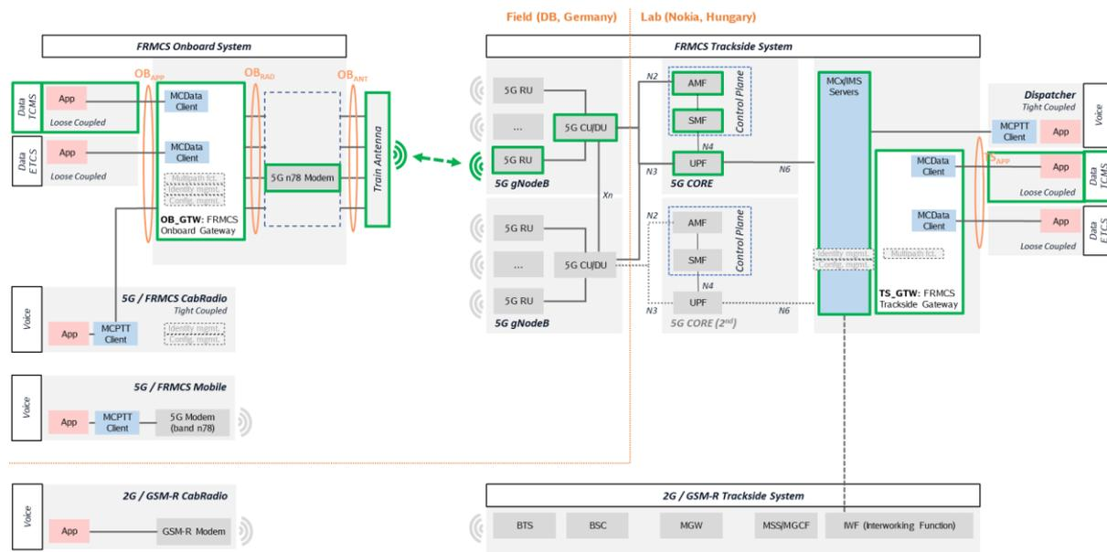
Figure 86: Architecture for test case TCMS\_TC\_001 (TC\_001a) (Testbed Germany)
