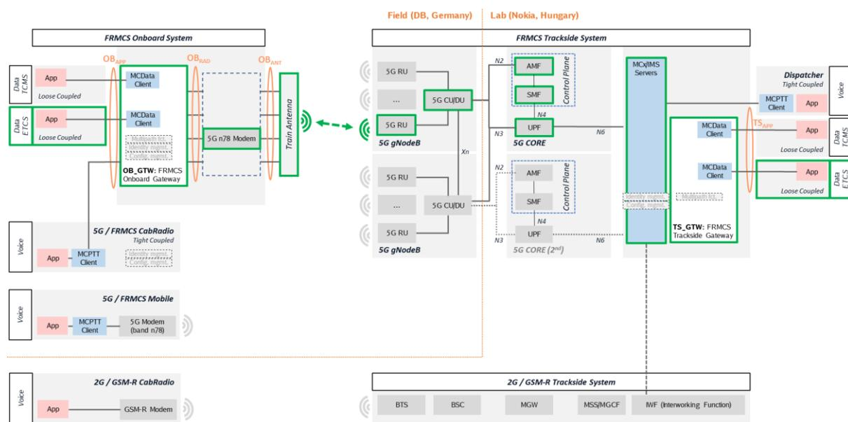
Figure 58: Architecture for test case ETCS\_WP3-WP5\_TC\_001 (Testbed Germany)
