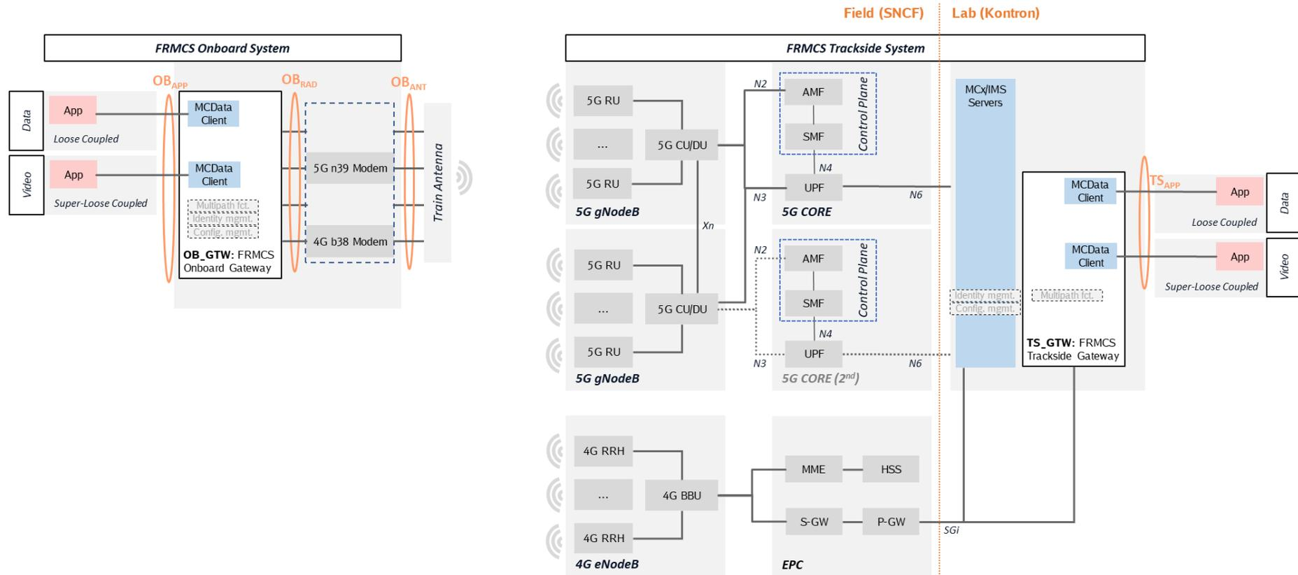
Figure 39: End-to-end test architecture of WP5 used for the field campaigns in the 5GRAIL Testbed France
