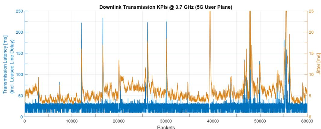
Figure 24: 5G user plane latencies and jitter in Downlink measured betw. trackside gateway and on-board switch during a drive test (excl. application processing delays)
