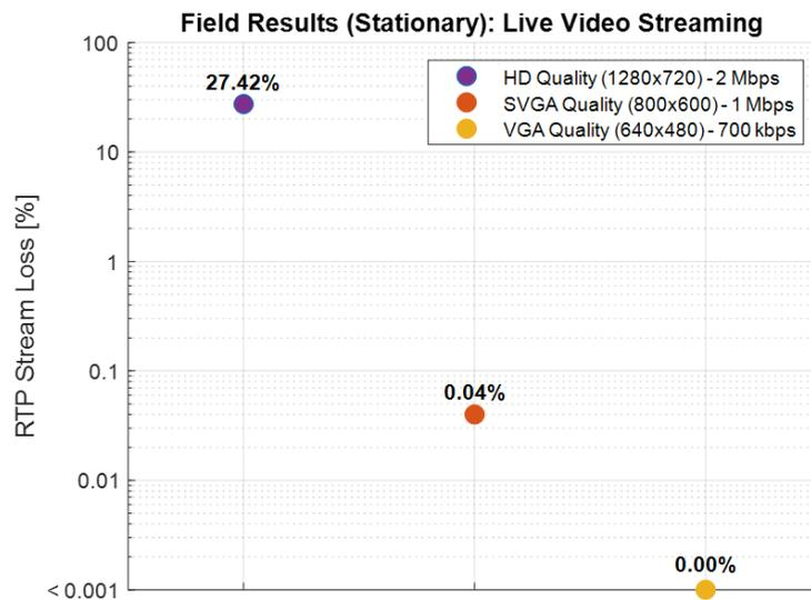
Figure 102: Comparison of different resolutions in Video Streaming Stationary Test (Testbed Germany)
