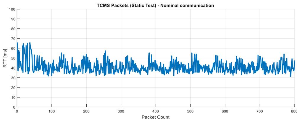
Figure 88: RTT for TCMS Static Tests, Test Case No. TCMS\_TC\_001 (TC\_001a) (Testbed Germany)
