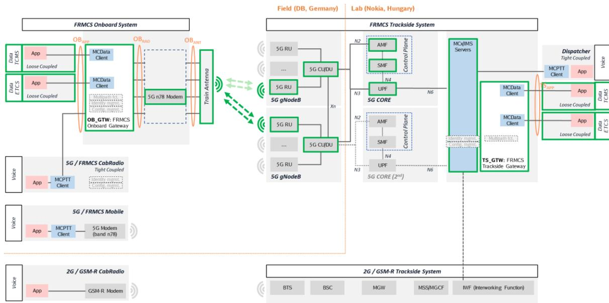
Figure 77: Architecture for test case ETCS\_WP3-WP5\_TC\_004, with intra- and inter-gNodeB handover (Testbed Germany)
