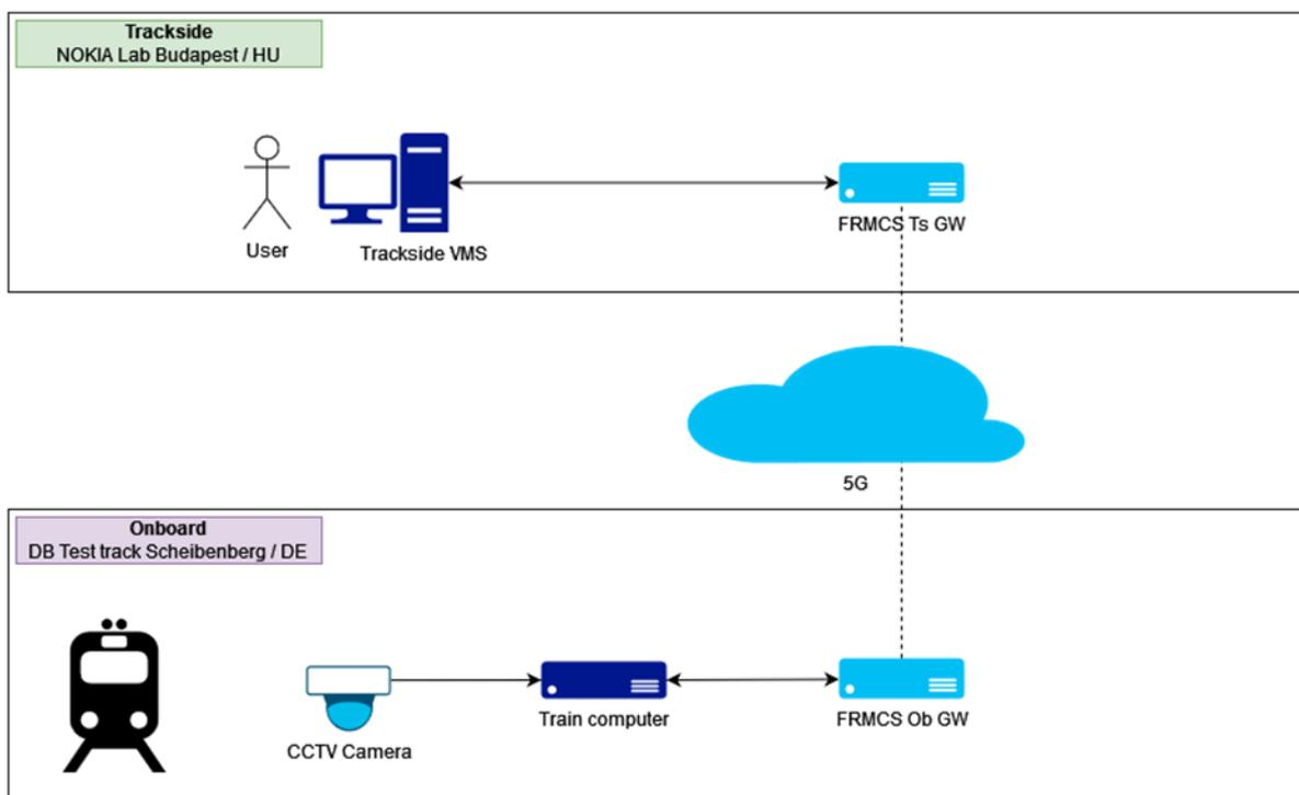
Figure 91: Test setup for the CCTV video field trials (Testbed Germany)
