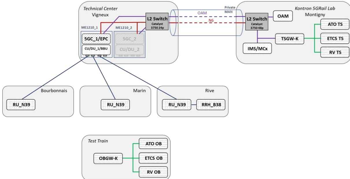
Figure 29: 5G architecture configuration A (Testbed France)
