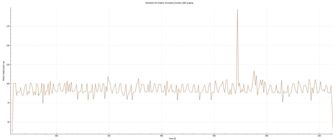
Figure 74: RTT for ETCS Dynamic Tests with increased traffic, captured in trackside traces (RBC), Test Case No. ETCS\_WP3-WP5\_TC\_003 (Testbed Germany)
