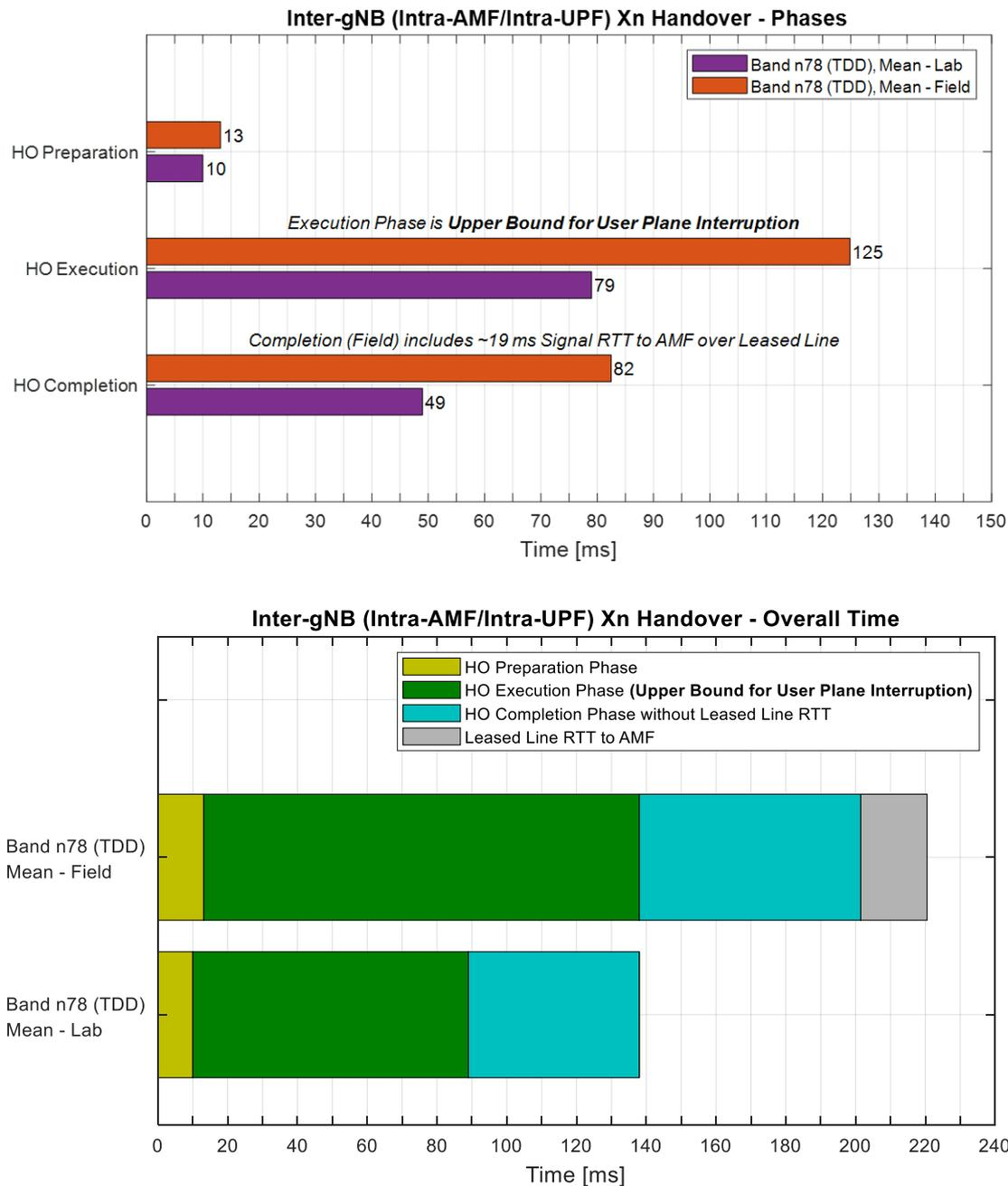
Figure 23: Comparison of control plane latencies in Xn-based Inter-gNB Intra-AMF HO for field conditions (Testbed Germany) vs. lab conditions (Lab Hungary)
