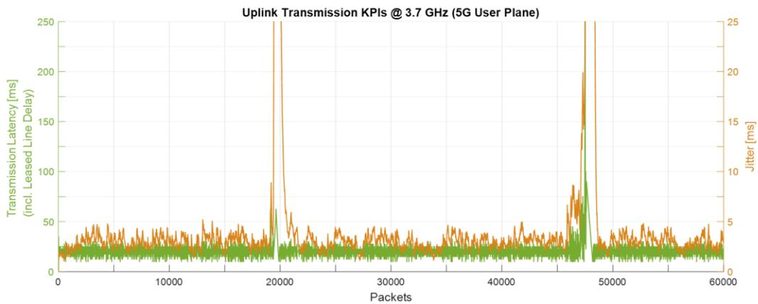
Figure 25: 5G user plane latencies and jitter in Uplink measured betw. on-board switch and trackside gateway during a drive test (excl. application processing delays)
