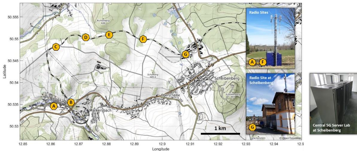
Figure 7: Layout of the 5G radio access network in the Testbed Germany
