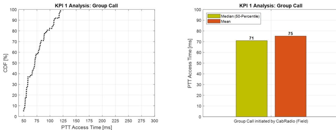
Figure 47: Statistical analysis of PTT Access Times for MCPTT group voice calls (Testbed Germany)
