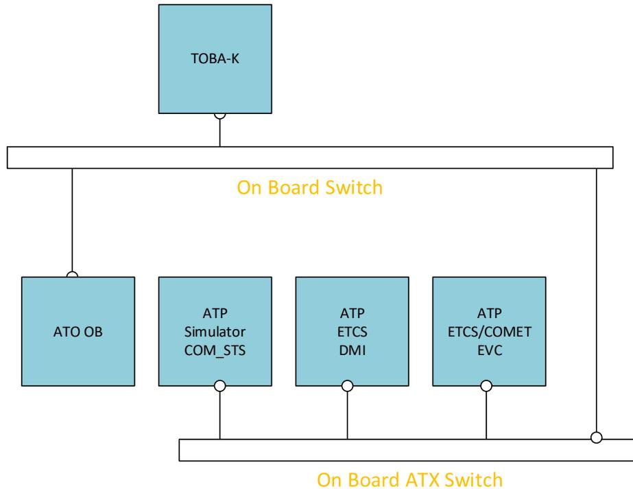
Figure 33: On-board equipment connections used in Testbed France
