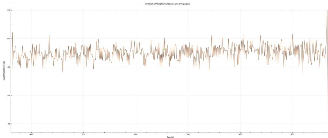
*Figure 78: RTT for ETCS in Combined Application Static Tests, captured in onboard traces (EVC), Test Case No. ETCS\_WP3-WP5\_TC\_004 (Testbed Germany)*
