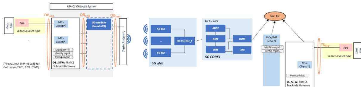
Figure 117: Involved OBApp and TSApp Interface (circled in light red) for ATO app. integration (Testbed France)
