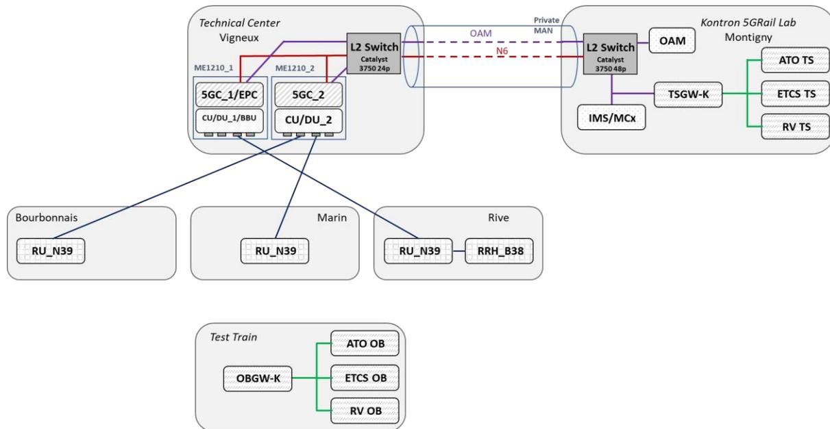
Figure 30: 5G architecture configuration B (Testbed France)
