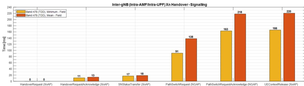
Figure 21: Measured times of the signalling information in different handover phases during Xn-based HO (analysis based on 120 handover records)
