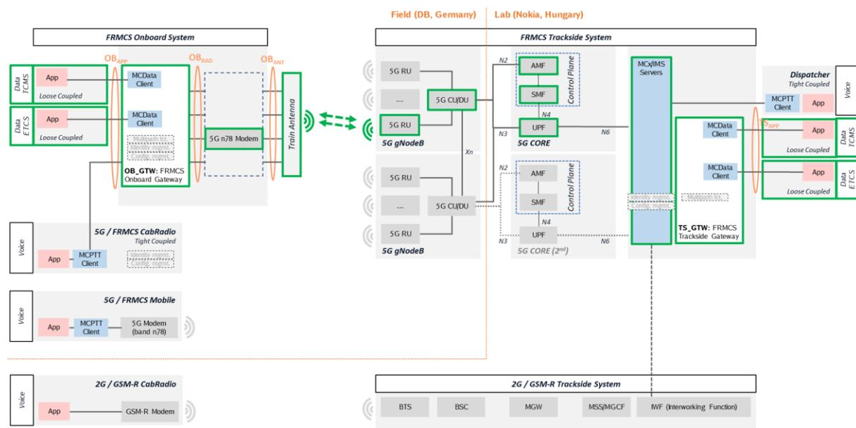
Figure 76: Architecture for test case ETCS\_WP3-WP5\_TC\_004 (Testbed Germany)
