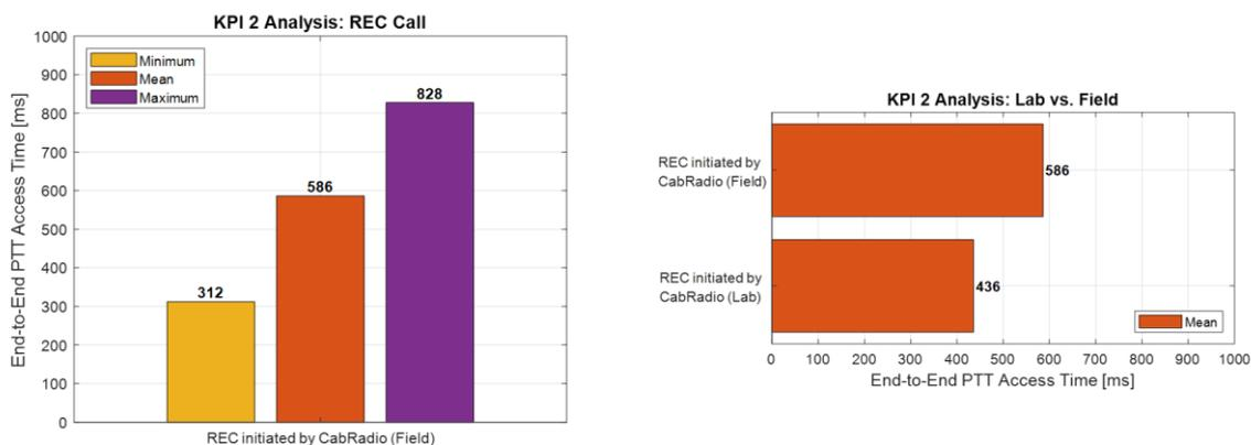
Figure 53: Statistical analysis of End-to-End PTT Access Times for MCPTT railway emergency calls and comparison of field vs. lab performance results (Testbed Germany)
