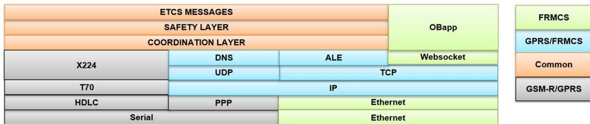
Figure 56: Evolution of the ETCS protocol stack for FRMCS.
