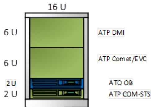
Figure 36: Rack implementation for ETCS/ATP over FRMCS tests (Testbed France)
