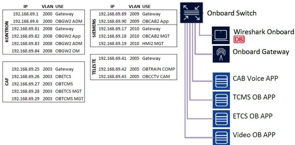
Figure 13: High-level on-board network design and IP plan (Testbed Germany)
