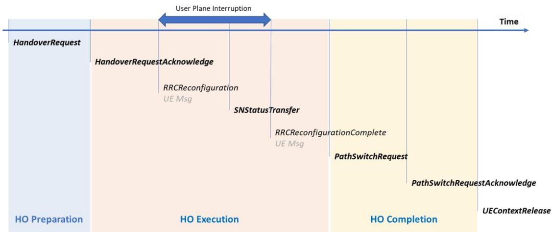
Figure 20: Phases and signalling information of Xn-based HO in 5G acc. to Appendix 14.1
