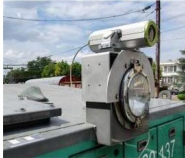
Figure 128: Frontal camera of the remote vision application (Testbed France)
