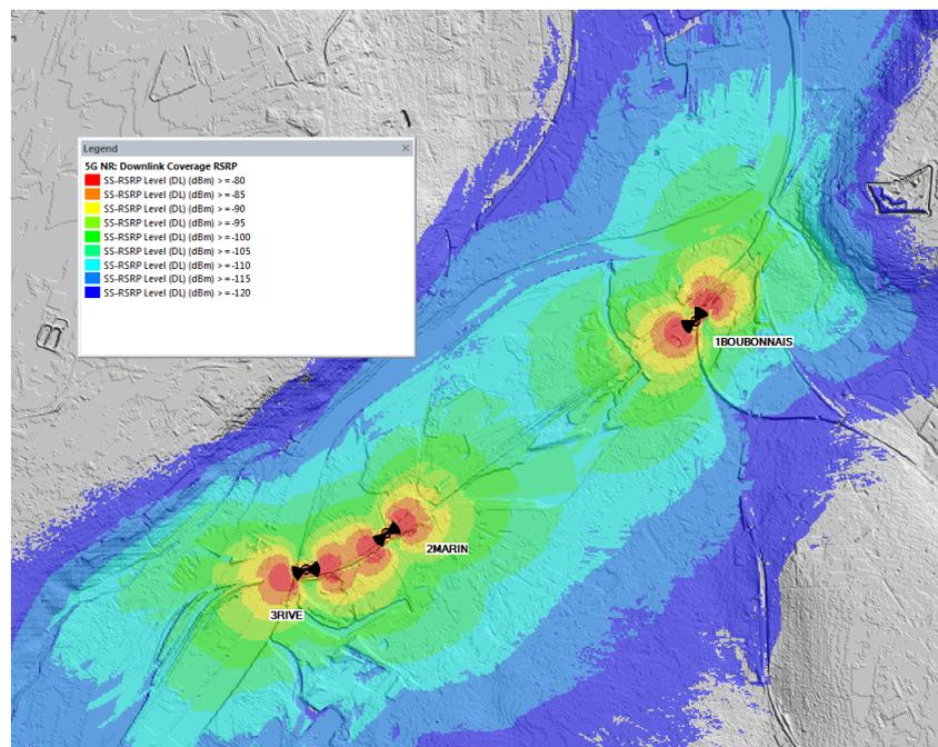
Figure 37 – RSRP Downlink Coverage Simulation using N39 band
