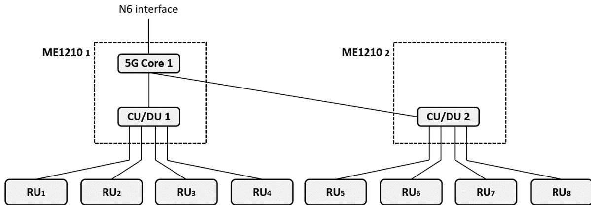
Figure 122: Configuration for inter gNode-B HO under the same 5G Core (Ref.D4.2 [10])
