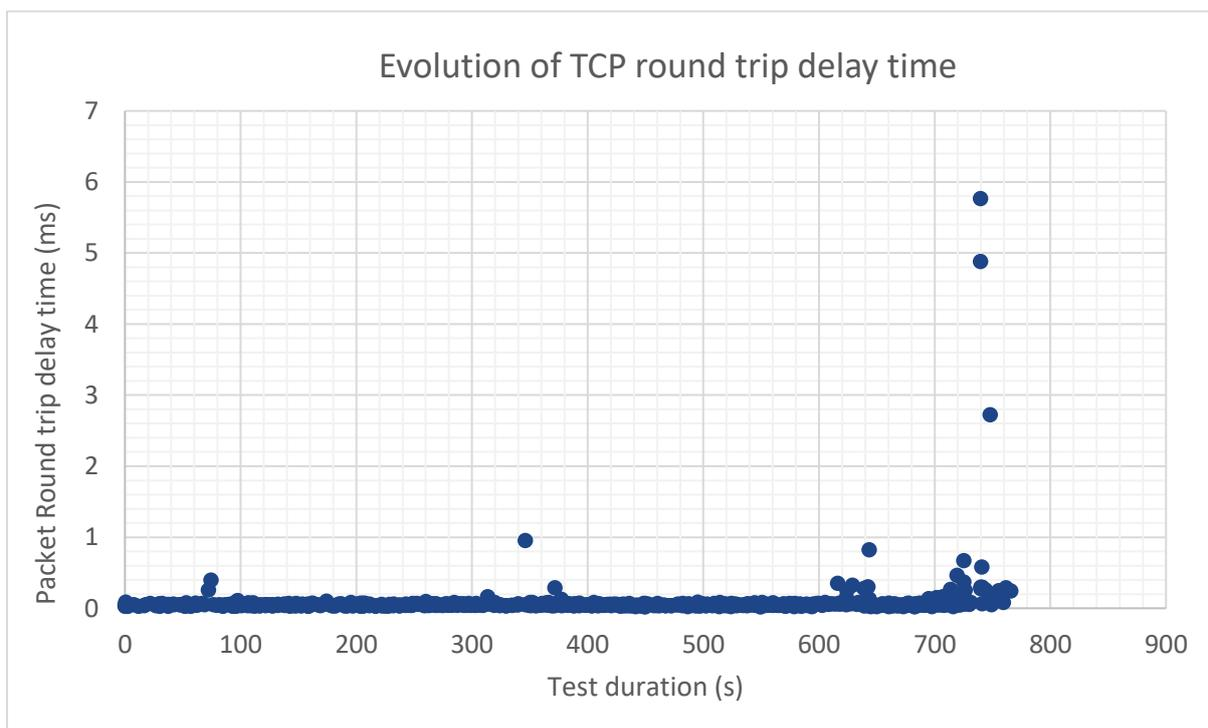
**Inter-gNodeB HO:** The communication is established, there is no interruption (application data loss) until the loss of 5G signals. This test was passed in both static and dynamic conditions. Wireshark traces are saved and shows a consistent exchange. During this test, both ATO and ATP were using the same network with dedicated communications in parallel.
