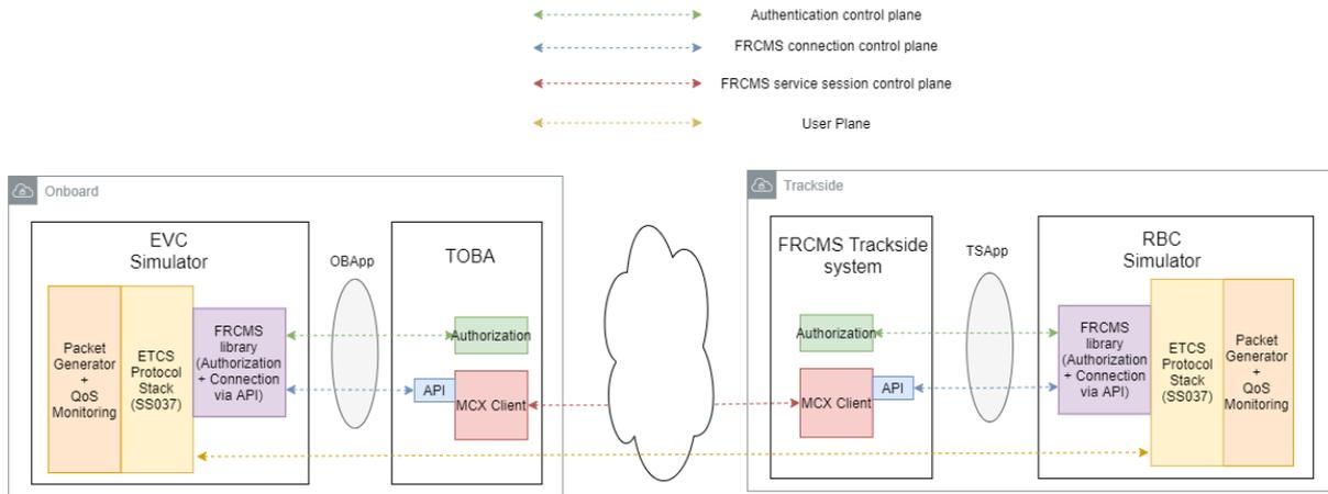
Figure 55: ETCS prototype architecture (provided by CAF)
