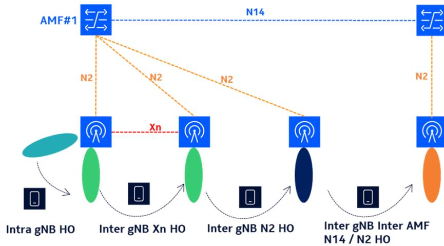
Figure 11: General overview of 5G handover situations, using one or two AMFs [8]
