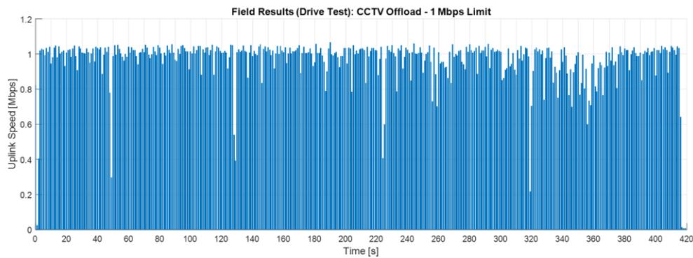
Figure 112: CCTV Offload performance in a dynamic setup (7 min drive test) with 1 Mbps offload speed limitation, Test Case No. CCTV\_TC\_001
