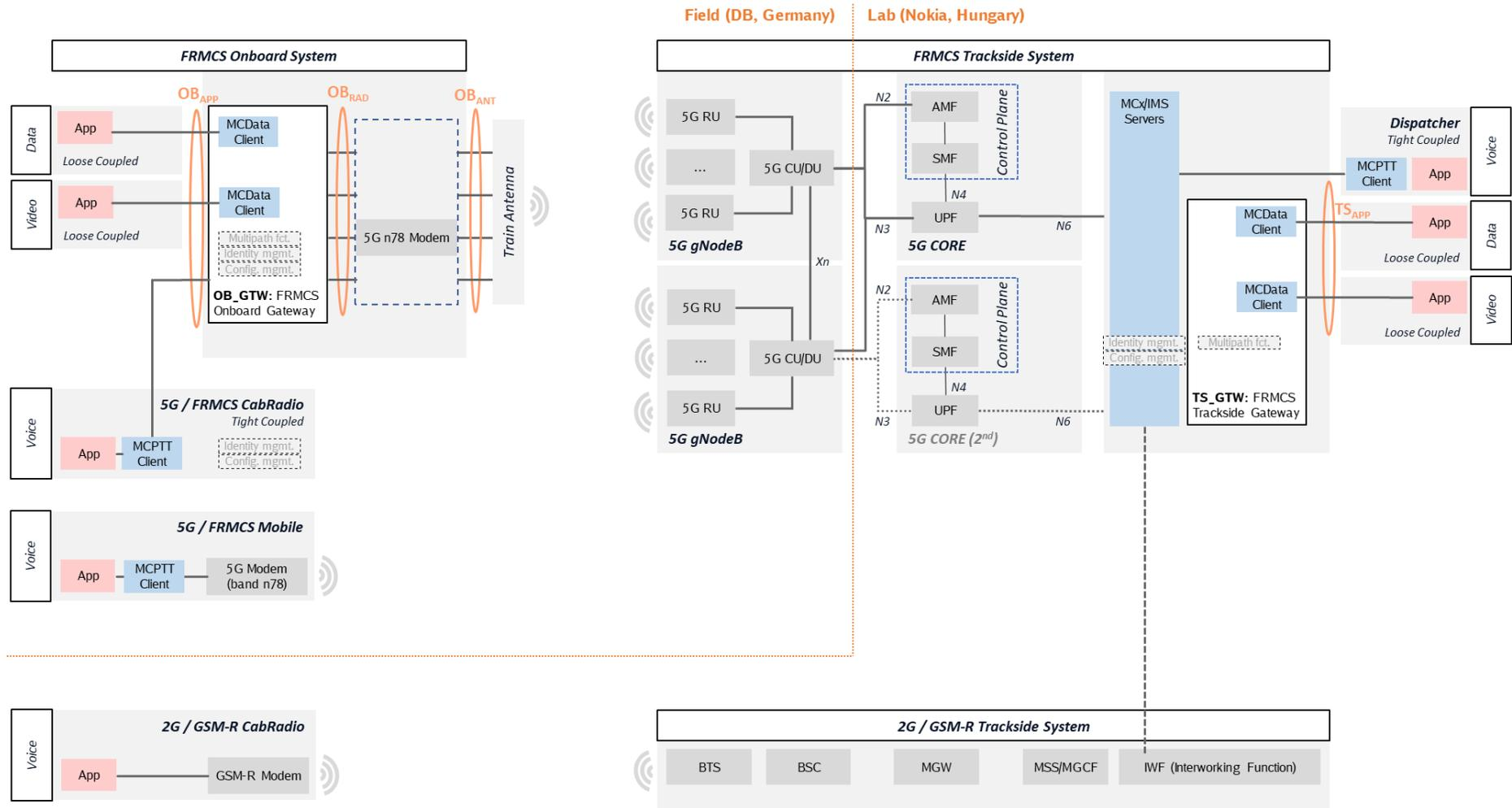
Figure 40: End-to-end test architecture of WP5 used for the field campaigns in the 5GRAIL Testbed Germany
