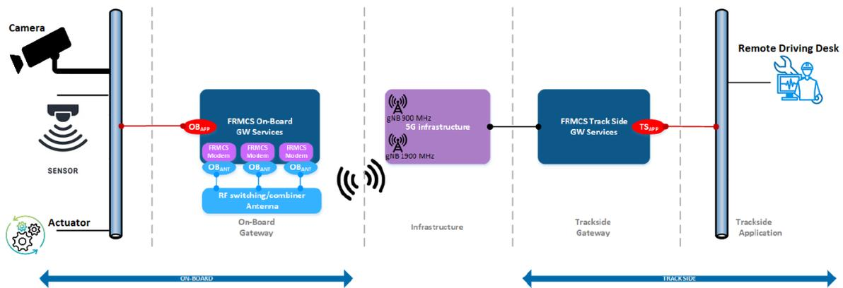
Figure 125: Global architecture of the remote driving system in the FRMCS
