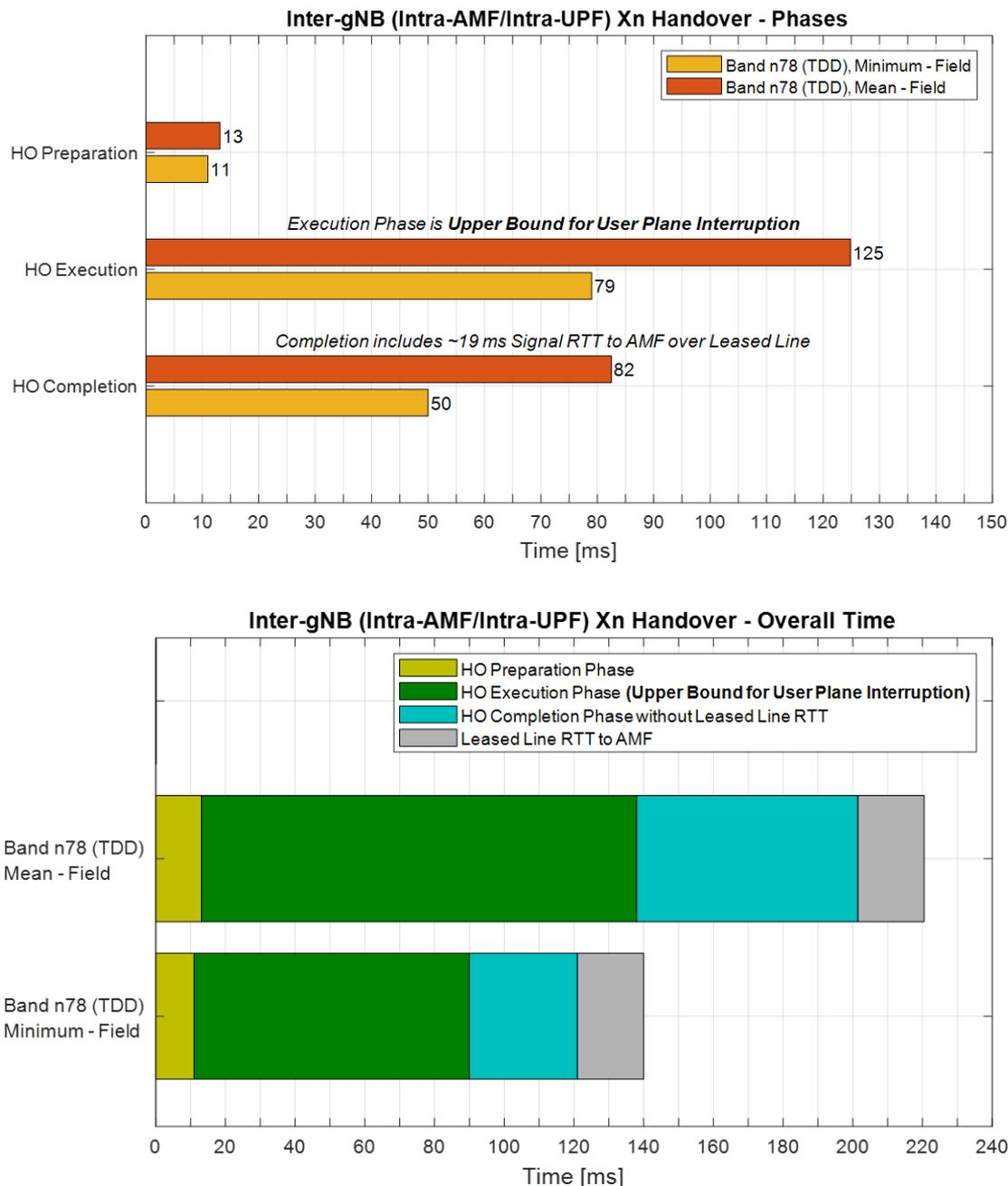
Figure 22: Control plane latencies in Xn-based Inter-gNB Intra-AMF HO (Testbed Germany)
