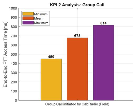
Figure 48: Statistical analysis of End-to-End PTT Access Times for MCPTT group voice calls (Testbed Germany)
