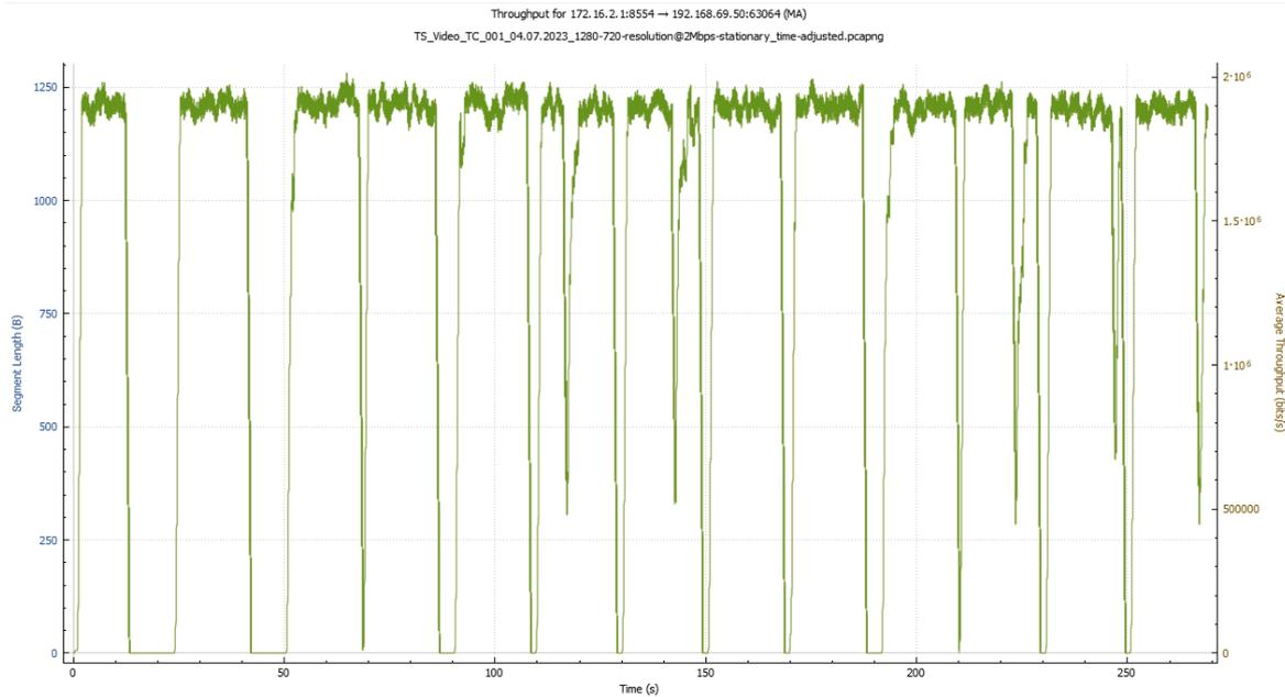
Figure 96: HD Video Streaming Stationary Test (Testbed Germany), throughput / goodput over time, Test Case No. Video\_TC\_001
