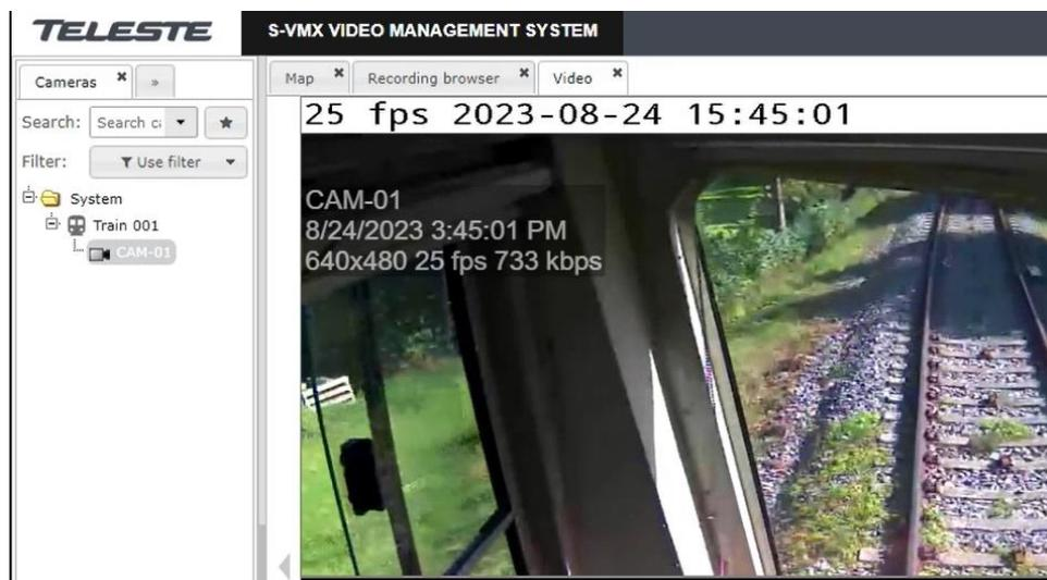
*Figure 108: VGA Video Streaming Drive Test (Testbed Germany), latency test showing same time stamps of onboard computer (transmitter side) and trackside server (receiver side), Test Case No. Video\_TC\_003*
