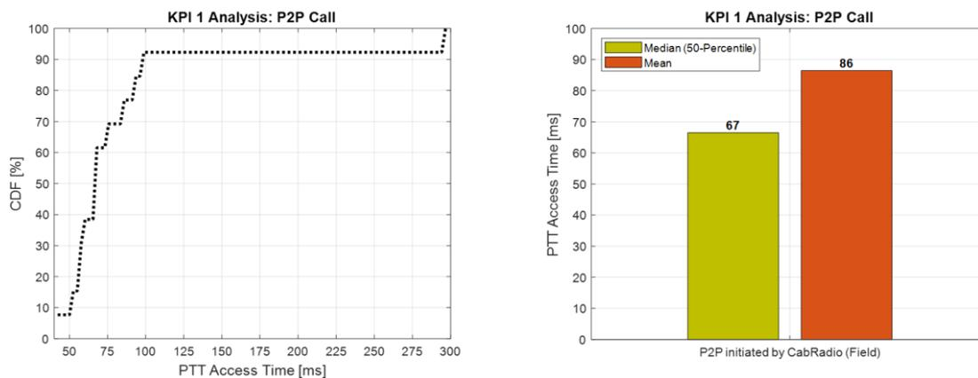
Figure 44: Statistical analysis of PTT Access Times for MCPTT point-to-point voice calls (Testbed Germany)
