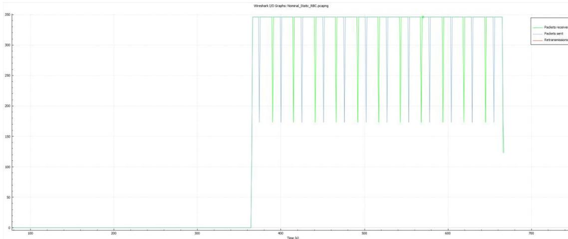
Figure 63: Packet Information (Sent/Received/Retransmissions) for ETCS Static Tests, captured in trackside traces (RBC), Test Case No. ETCS\_WP3-WP5\_TC\_001 (Testbed Germany)
