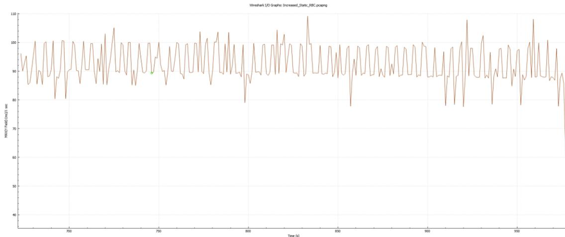
Figure 70: RTT for ETCS Static Tests with increased traffic, captured in trackside traces (RBC), Test Case No. ETCS\_WP3-WP5\_TC\_003 (Testbed Germany)
