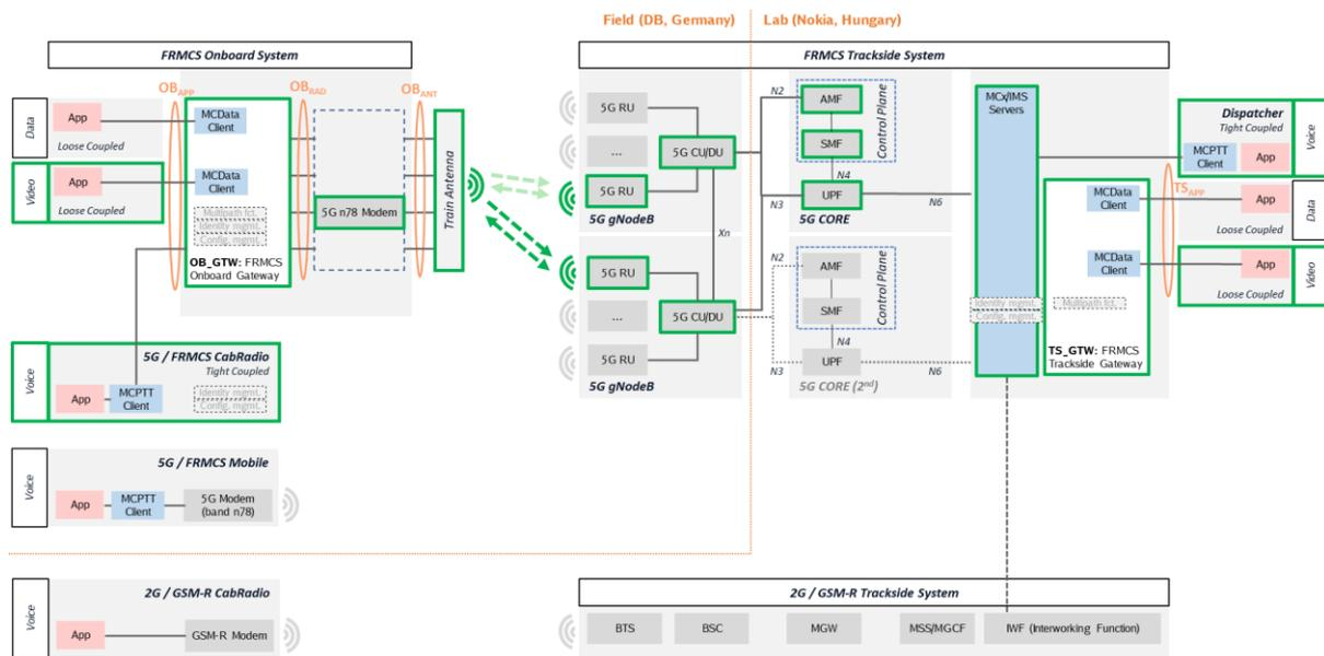
Figure 54: Architecture for test cases Voice\_017 (Testbed Germany)
