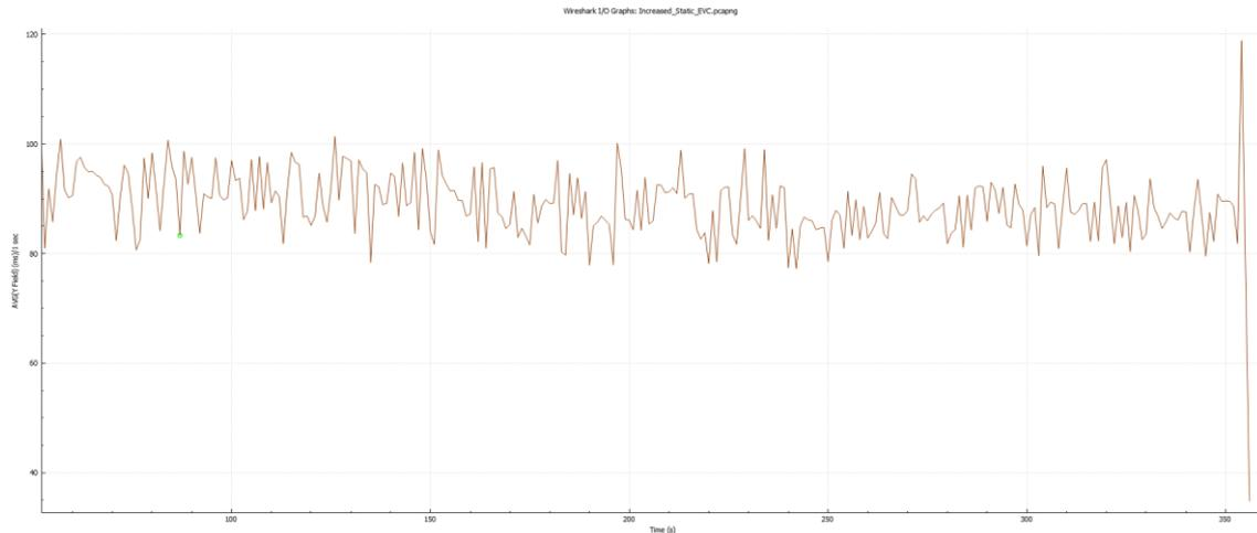
Figure 68: RTT for ETCS Static Tests with increased traffic, captured in onboard traces (EVC), Test Case No. ETCS\_WP3-WP5\_TC\_003 (Testbed Germany)
