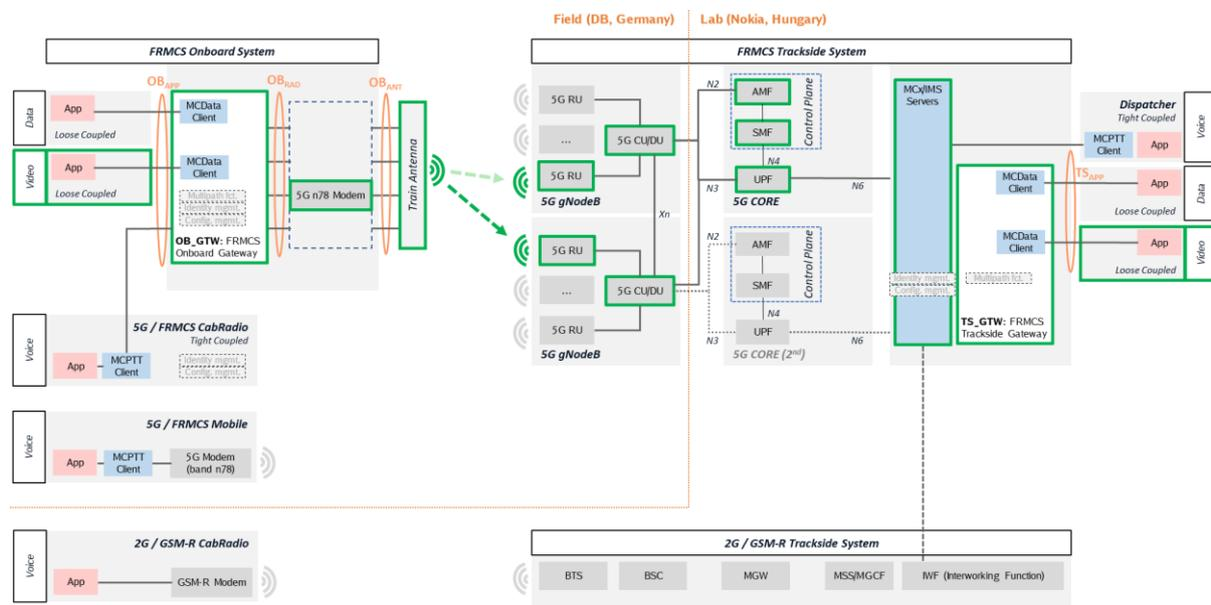
Figure 104: Architecture for test case Video\_TC\_003 (Testbed Germany)
