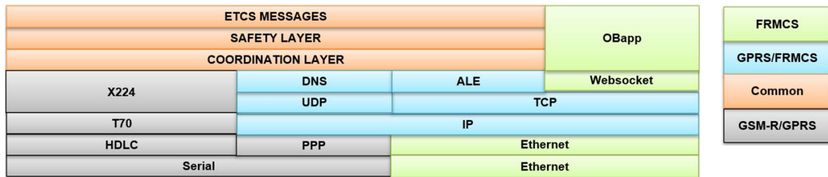
Figure 18: Evolution of the ETCS protocol stack for FRMCS (Ref. 5.1)
