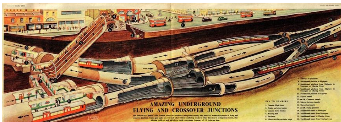
Figure 17: Multilevel tunnelling description [23]
