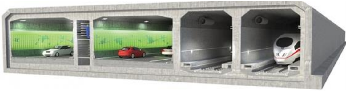
Figure 15: Examples of shared tunnel section [21]
