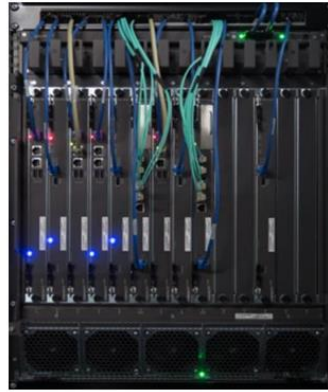
Figure 17: MCS-S and HLR 13U-14 slots ATCA platform
