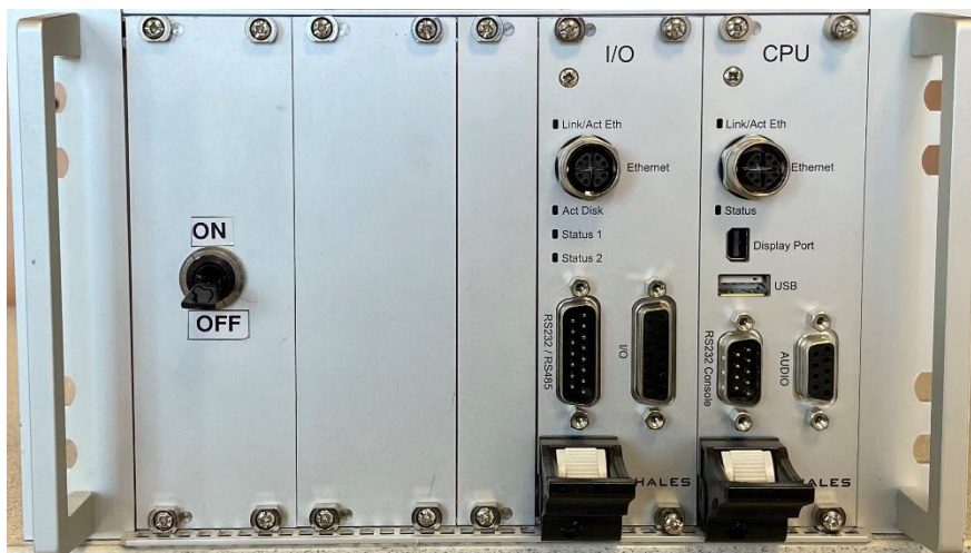
Figure 85: APIS on-board server (Front panel).
