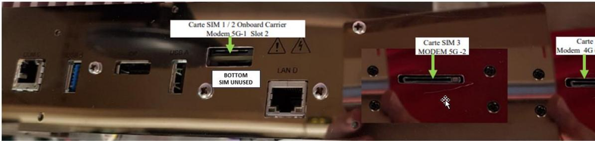
Figure 45: OnBoard Gateway SIM card locations
