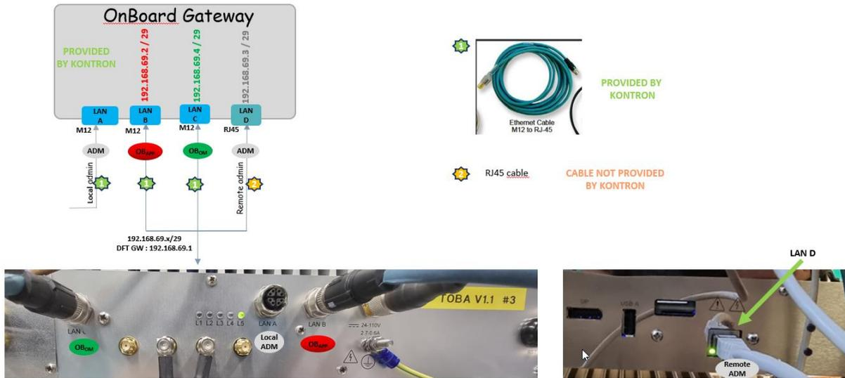
Figure 43: OnBoard Gateway Network interfaces
