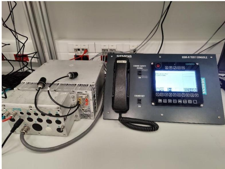
Figure 25: Siemens CAB radio in WP3 control room
