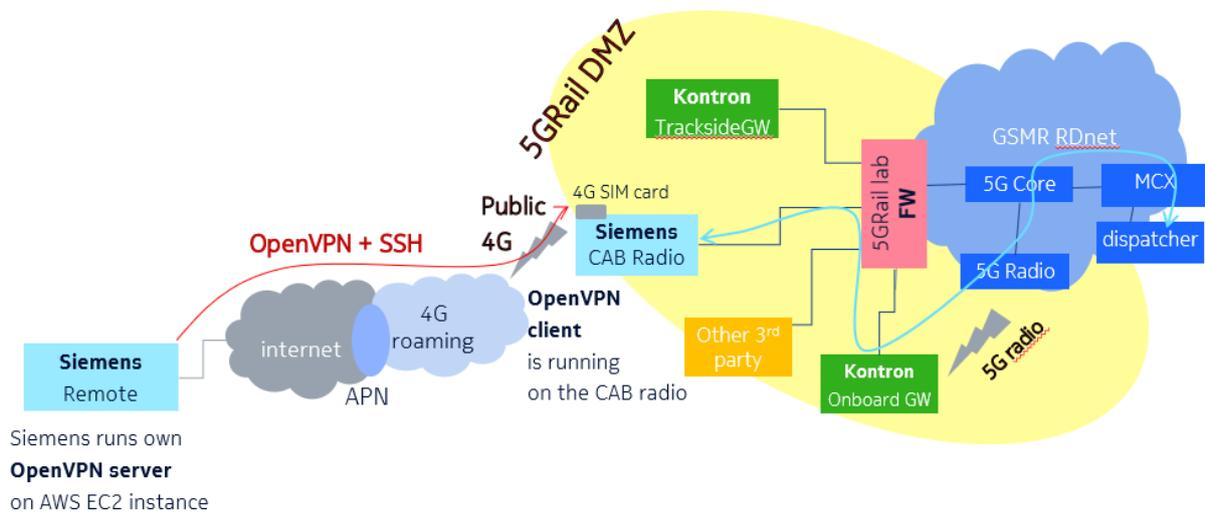
Figure 24: Remote access setup for Siemens
