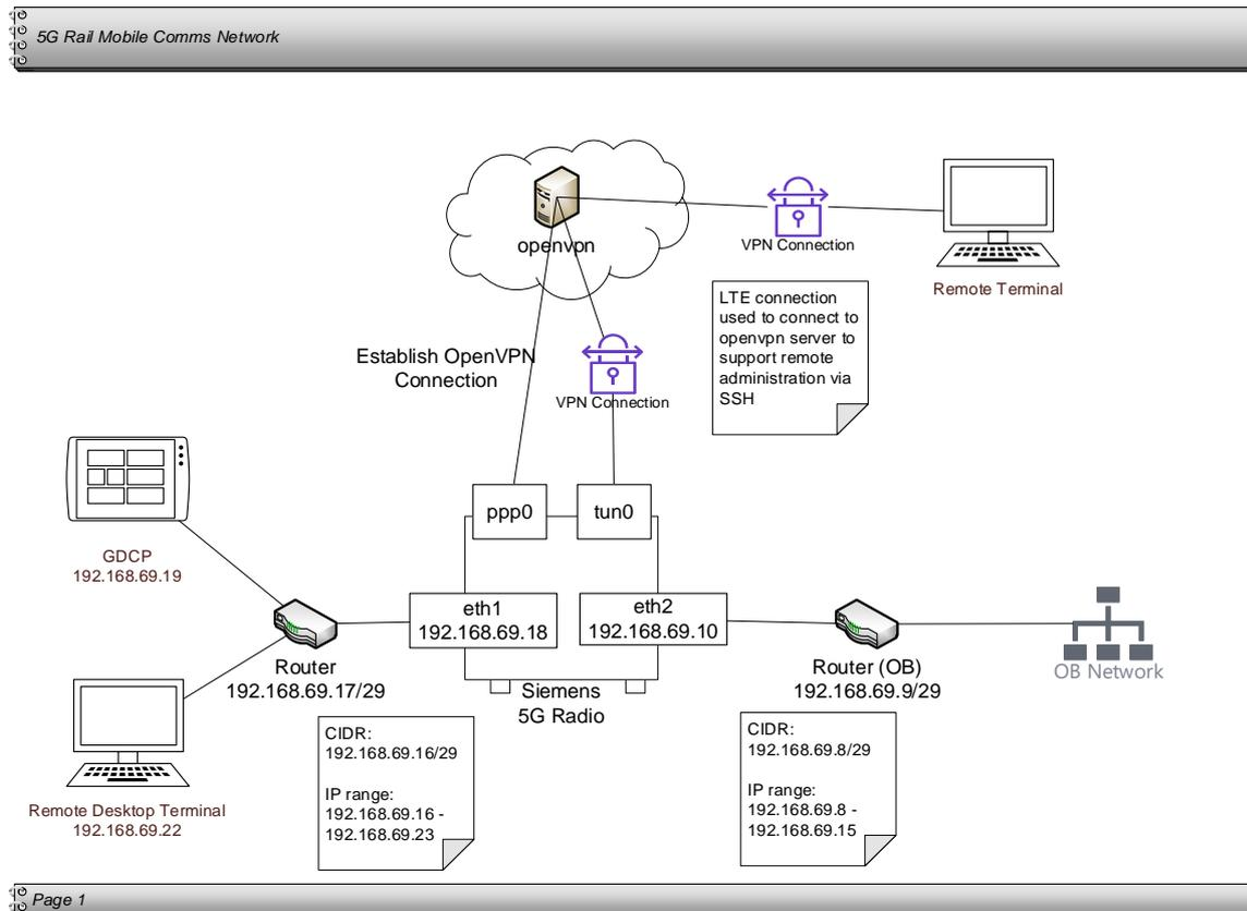
Figure 47: Network configuration of Siemens 5G CAB Radio
