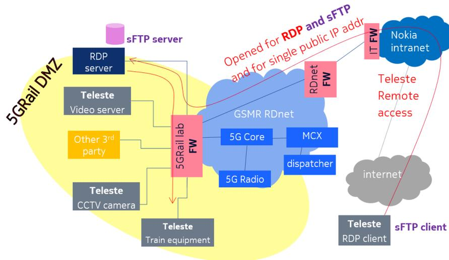
Figure 30: Remote access setup for Teleste
