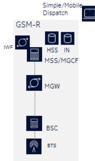
Figure 15: GSM-R configuration
