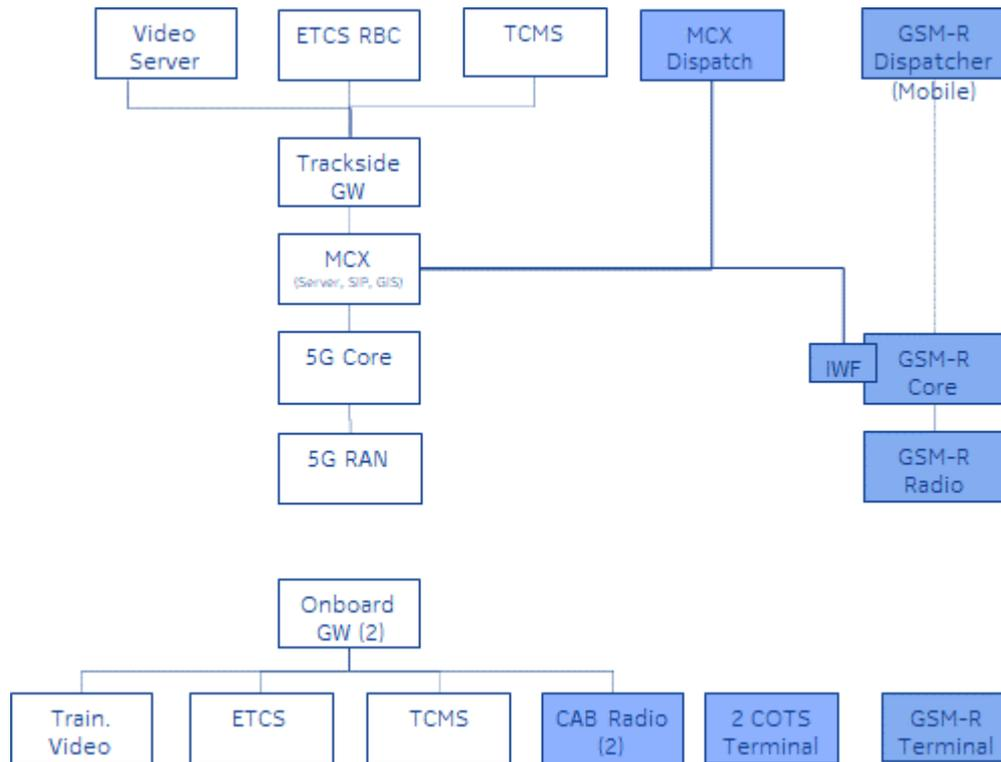
Figure 14 Connectivity Overview GSM-R Interworking
