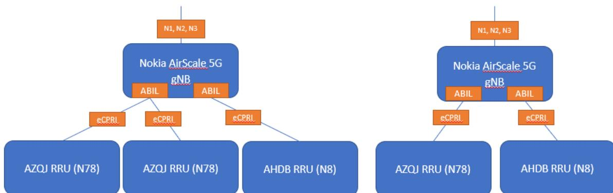
Figure 4: 5G radio configuration
