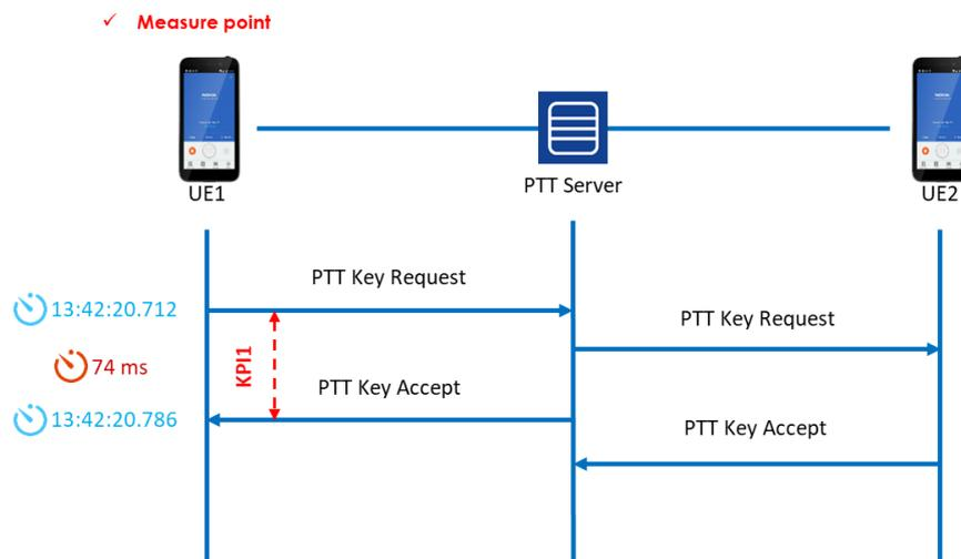
**Figure 37: MCX KPI 1 Measurement Configuration**
