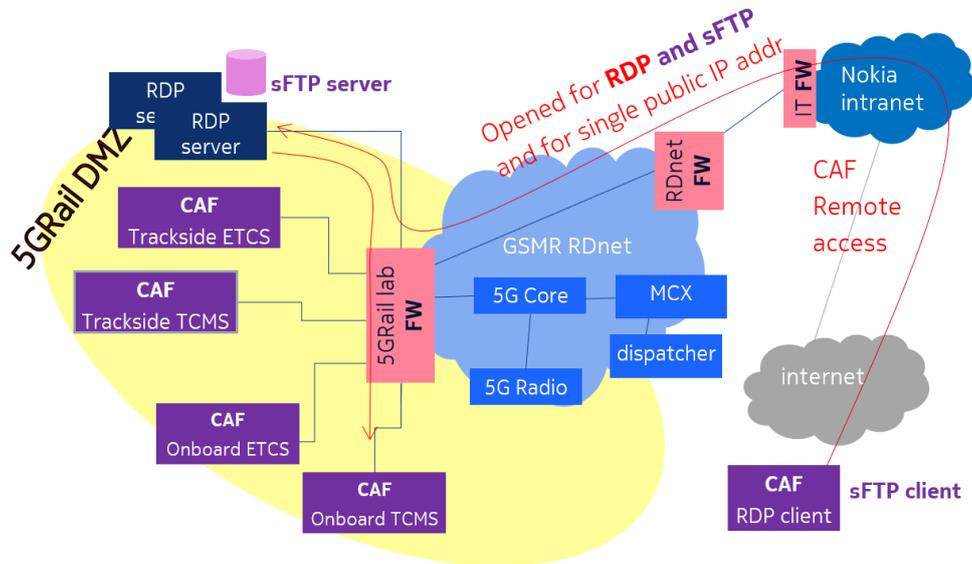
Figure 27: Remote access setup for CAF
