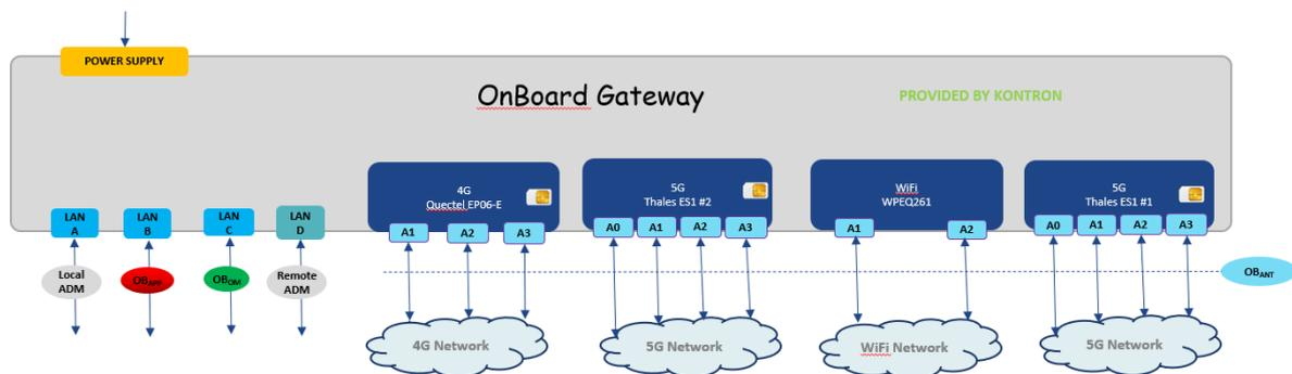
Figure 41: OnBoard Gateway Hardware overview
