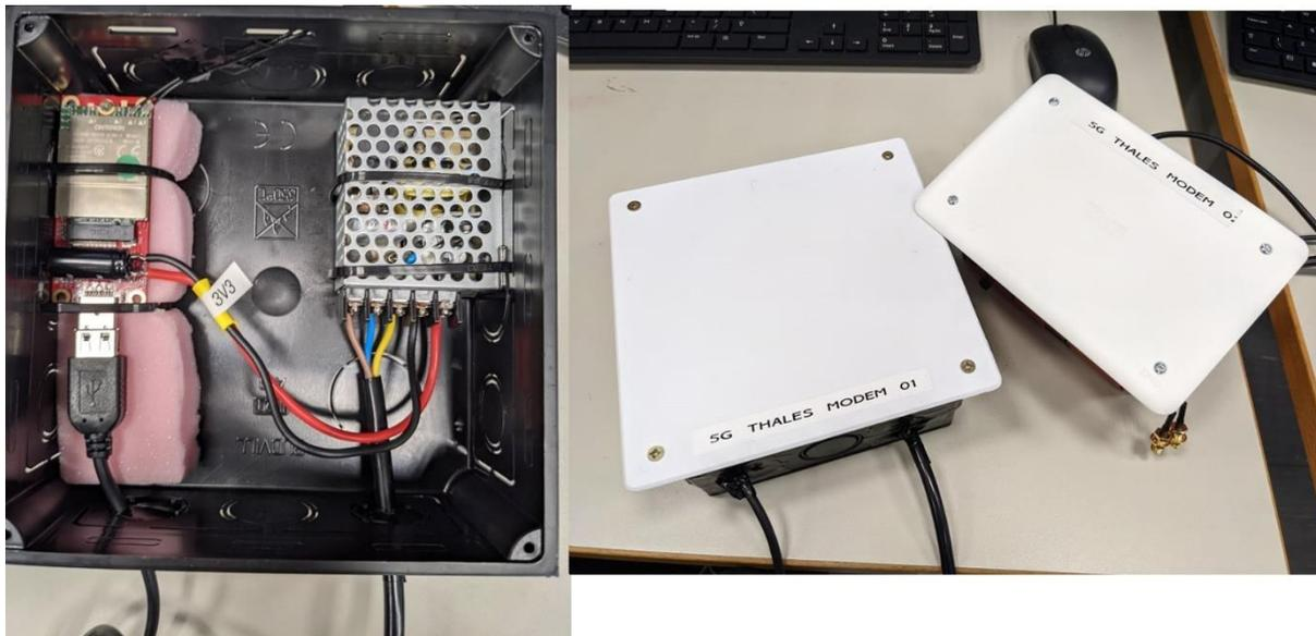
Figure 11: Picture from Thales modem
