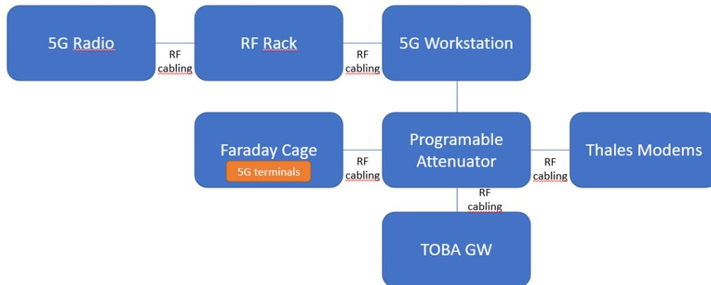
Figure 6: RF cabling configuration
