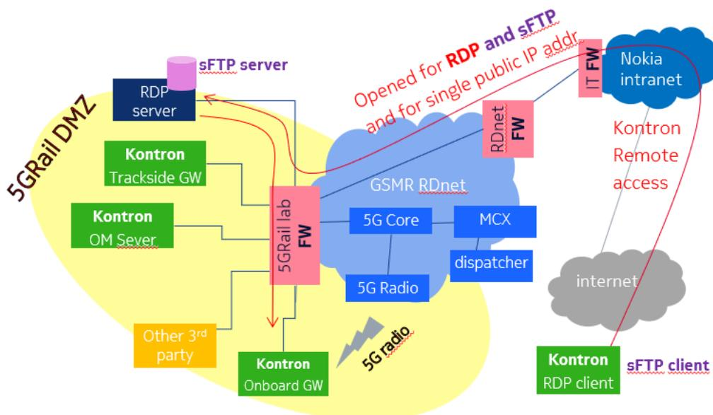
Figure 20: Remote access setup for Kontron
