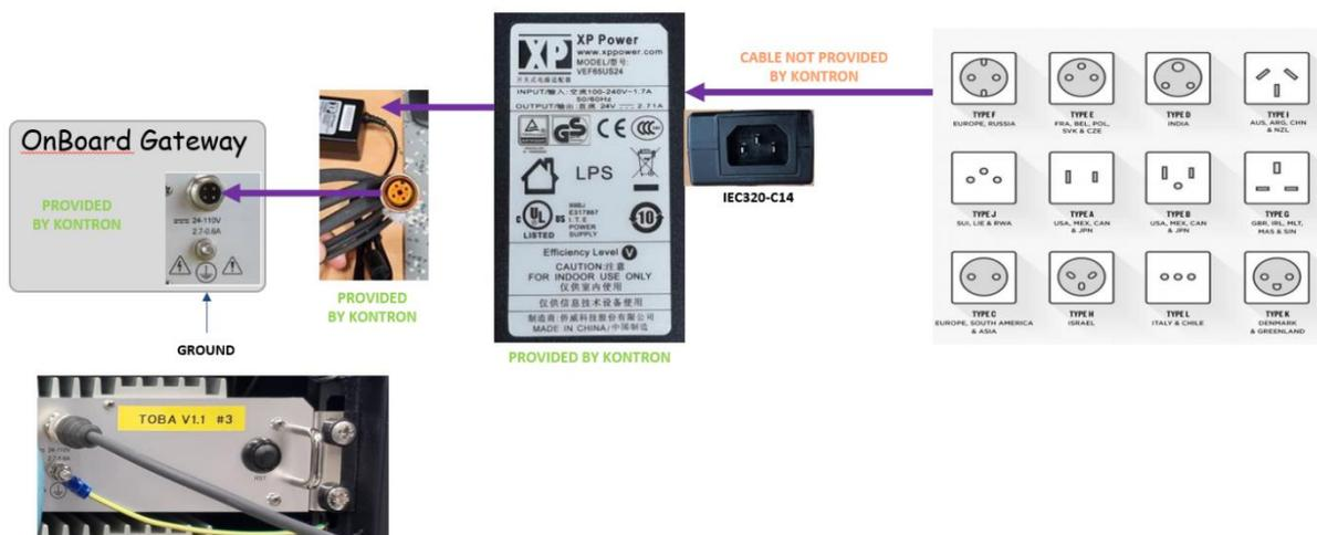
Figure 42: OnBoard Gateway Power connector
