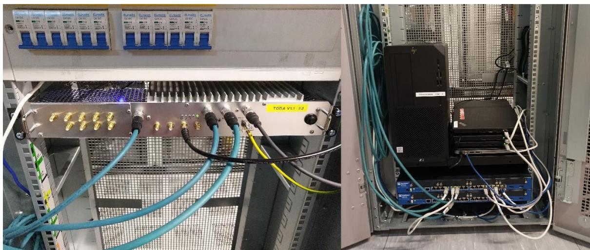
Figure 22: Onboard and Trackside gateways
