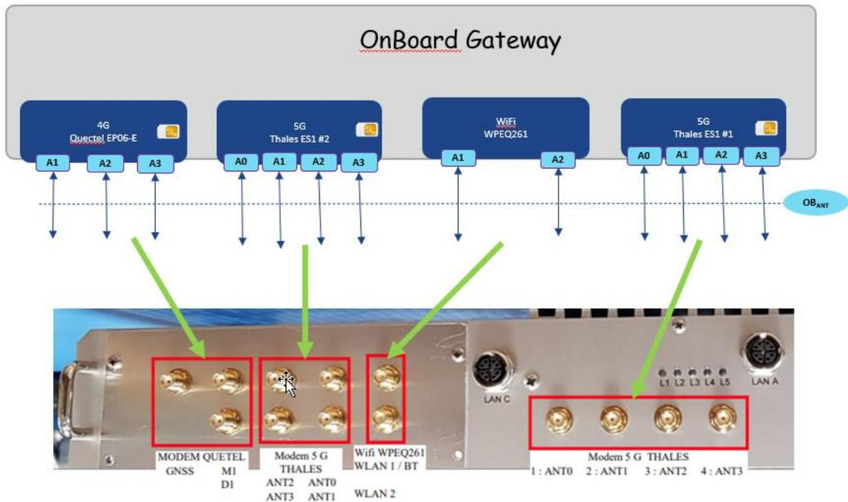
Figure 44: OnBoard Gateway Modem (antenna) interfaces
