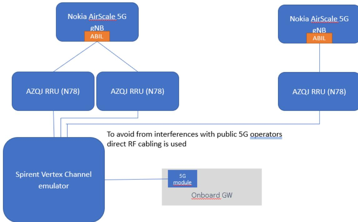
Figure 33: RF configuration setup with Spirent Vertex Channel Emulator
